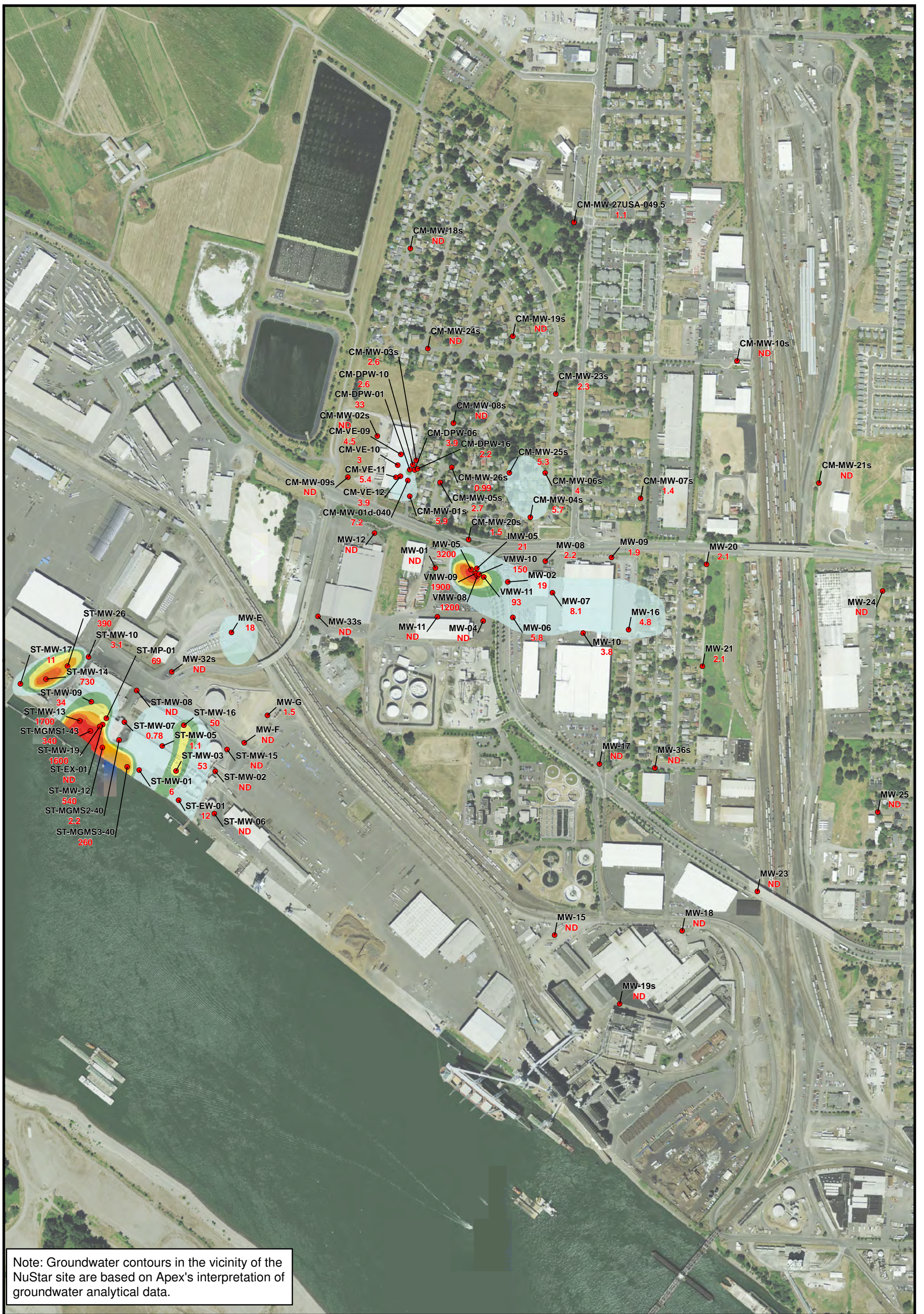
Figure 2-17 TCE Isoconcentrations in Shallow USA Zone Groundwater 1st Quarter 2013 Feasibility Study NuStar, SMC, and Cadet Vancouver, WA
