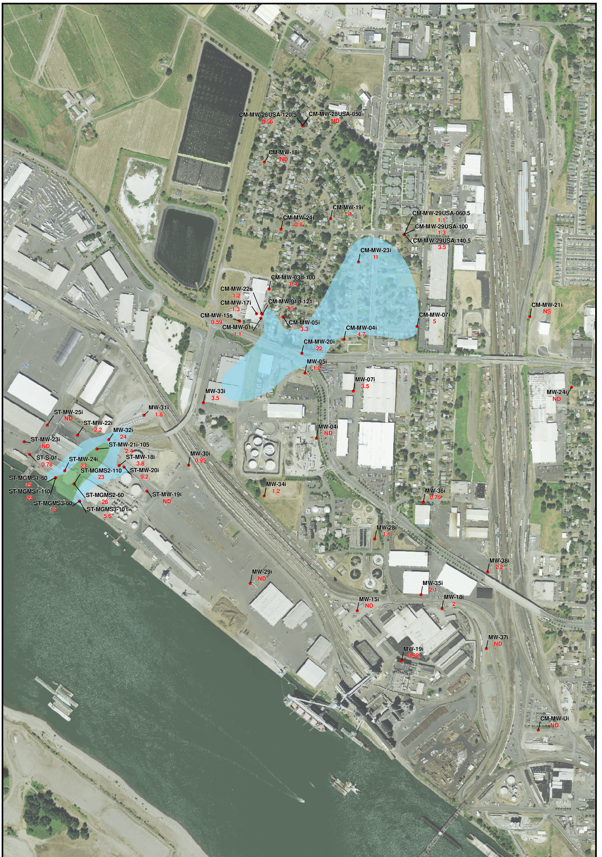
Figure 2-20 PCE Isoconcentrations in Intermediate USA Zone Groundwater 1st Quarter 2013
