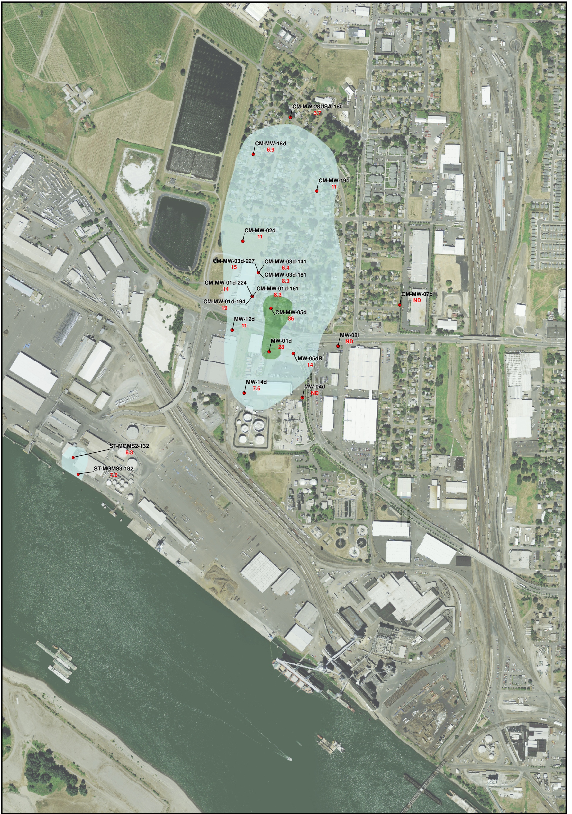
Figure 2-21 TCE Isoconcentrations in Deep USA Zone Groundwater 1st Quarter 2013
