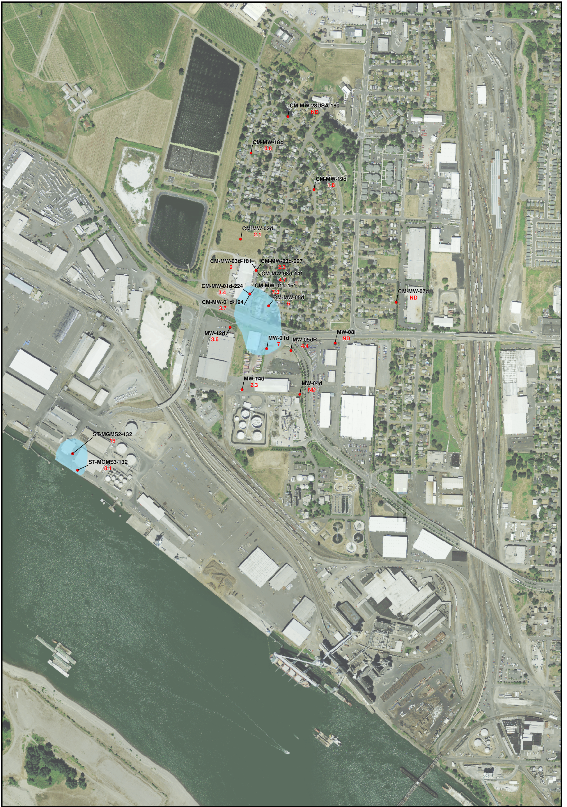
Figure 2-22 PCE Isoconcentrations in Deep USA Zone Groundwater 1st Quarter 2013
