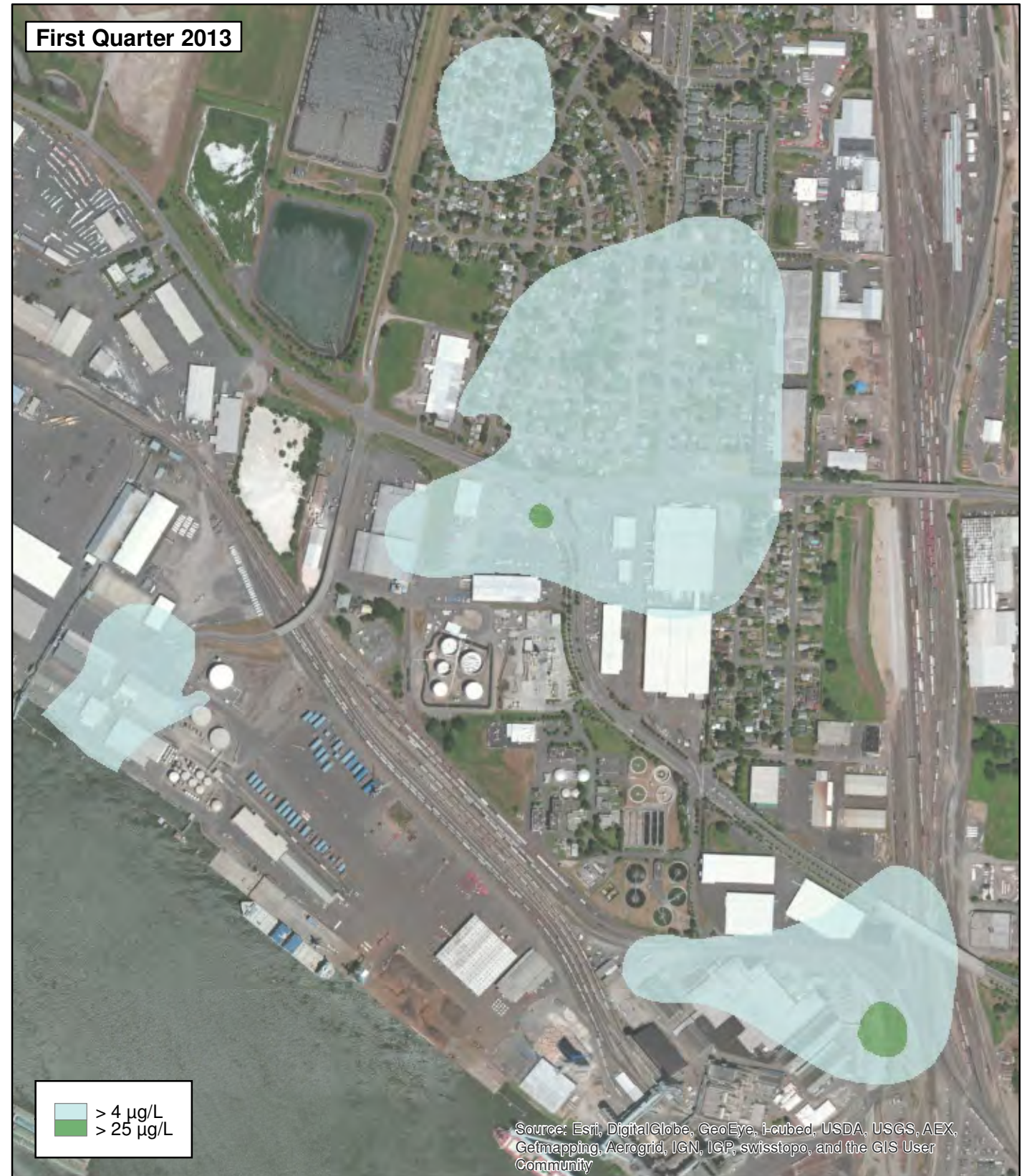
Figure 2-25 TCE Isoconcentrations in USA Intermediate Zone First Quarter 2009/First Quarter 2013
