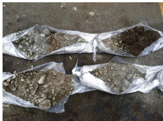
Photo #6: Continuous soil cores collected in plastic sheeting during borehole drilling.
