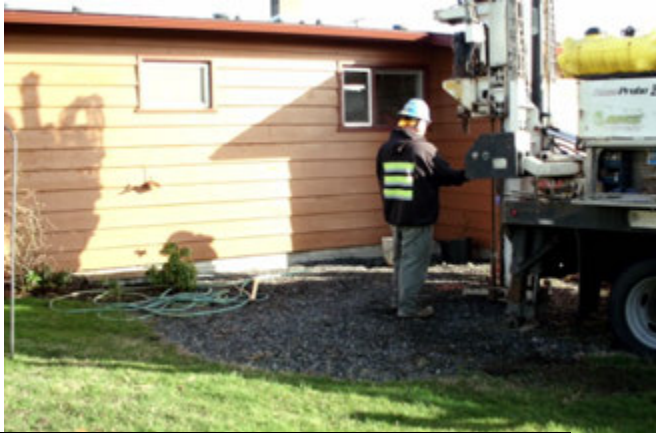
Photo #1: View of direct push probe drilling at boring B-1 – where former heating oil fuel tank was located. Note gravel surface area indicated area of excavation.
