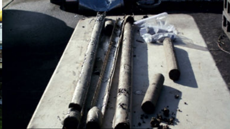
Photo #2: View of the typical soil encountered at the Site – stiff clay. These cuttings are from boring B-1.
