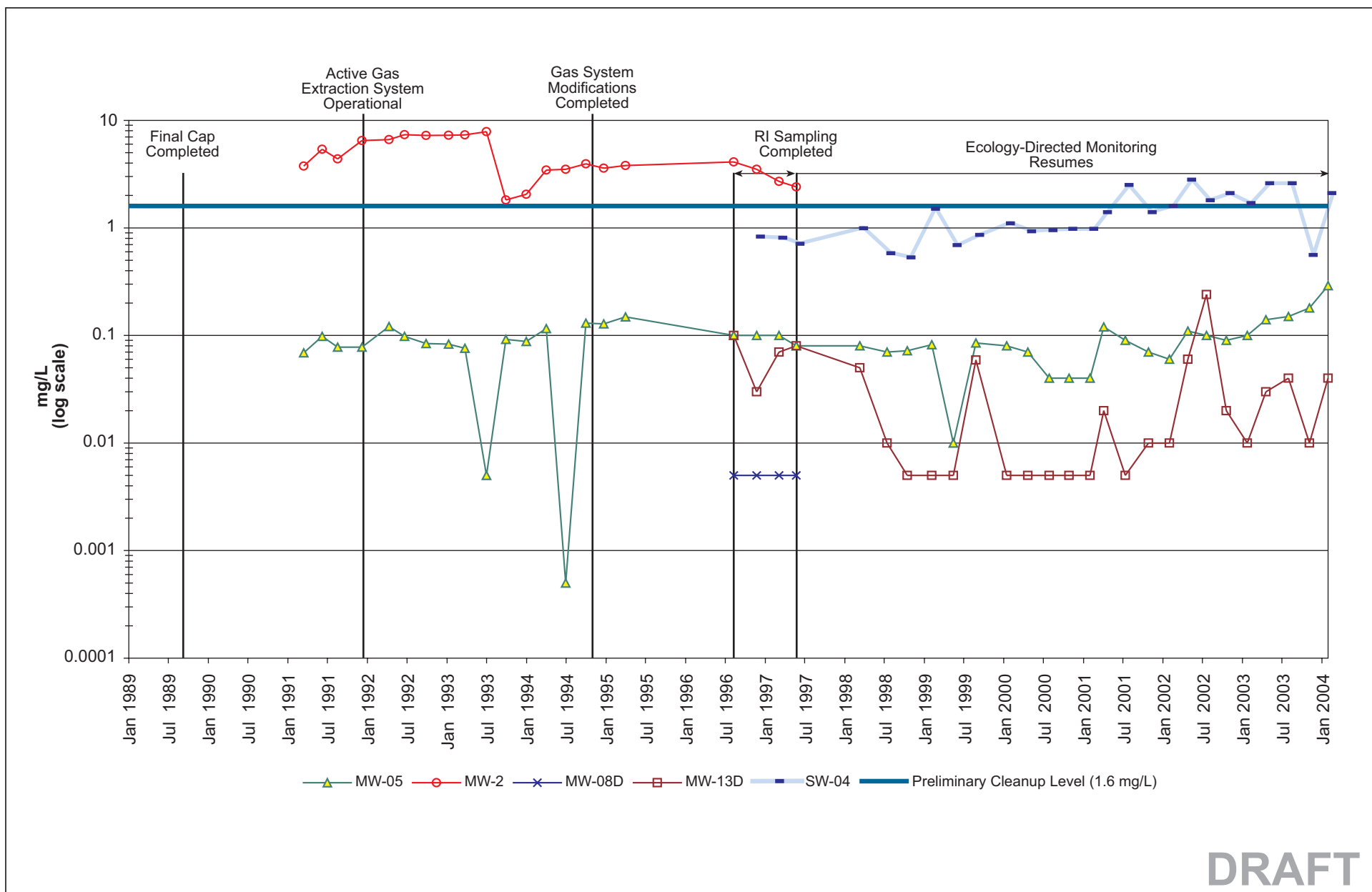
Figure 9-15b Time-Series Plot of Nitrate in Groundwater and Surface Water for the MW-02 to SW-04 Flow Path Hansville Landfill RI/FS
