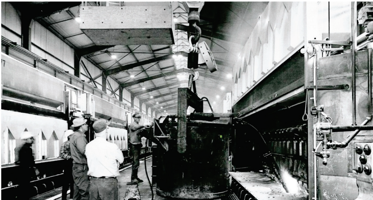
This photograph from the late 1960s shows one of the Reynolds “potlines” (the A-line in Room 51) during Longview plant operations.
