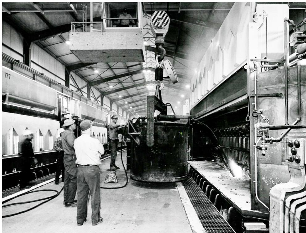
The diagram (top) illustrates the aluminum manufacturing or “reduction” process. Solid alumina is placed in a “pot” and dissolved in a cryolite solution (consisting of sodium, fluoride, and aluminum). Electricity is then passed through the material in the pot to produce molten aluminum. The photograph (bottom) from the late 1960s shows one of the Reynolds “potlines” (the A-line in Room 51) during Longview plant operations.
