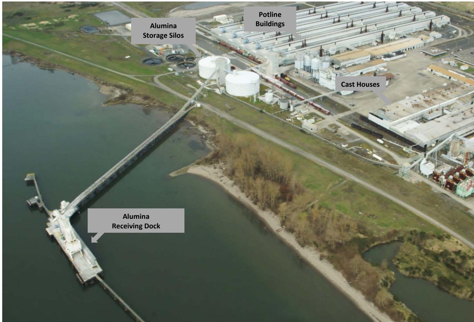
Alumina used at the Reynolds Facility was received by ship. The alumina was transferred to storage silos and then used in the potline buildings to produce molten aluminum (see Plate 2-3). The aluminum was then cast into solid form inside the cast houses. The aluminum manufacturing was curtailed in 2001, but the dock and storage silos remain in use for import of bulk products, including alumina required by the operating aluminum facility in Wenatchee.
