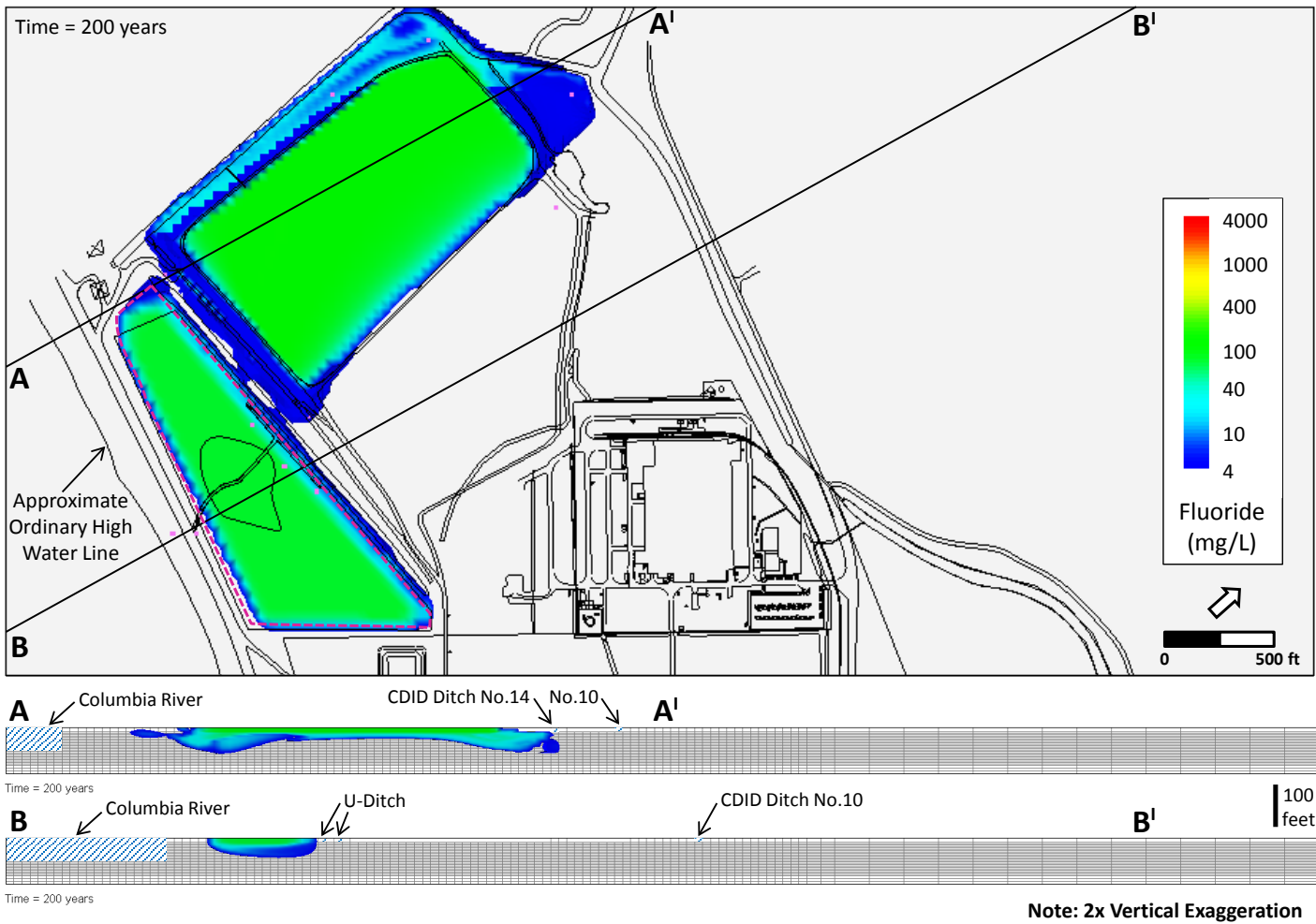
Figure 24 Plan View and Vertical X-sections of the Simulated West Groundwater Area Fluoride Plume after 200 Years with 50% Reduction in Infiltration
