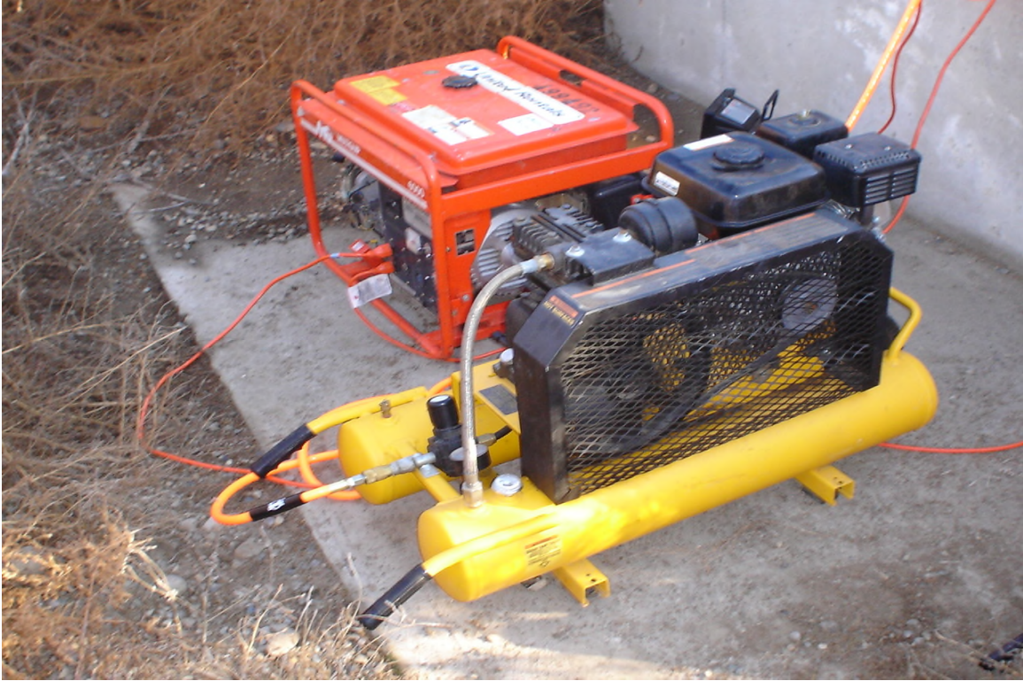
5-HP air compressor and generator setup.
