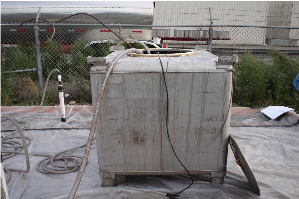
Stainless steel tank for mixing of sodium acetate, disodium phosphate, and water.
