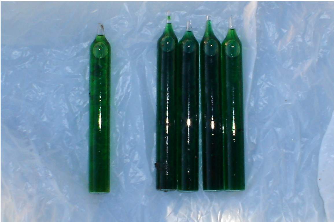
Ammonia test kits for groundwater collected from MW-4 and IW-1 through IW-4.
