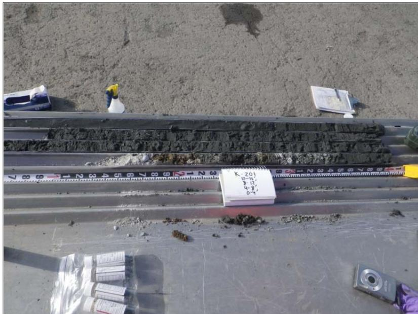
Figure 5-2. Soil Probe K-201 next to the former machine shop. .
