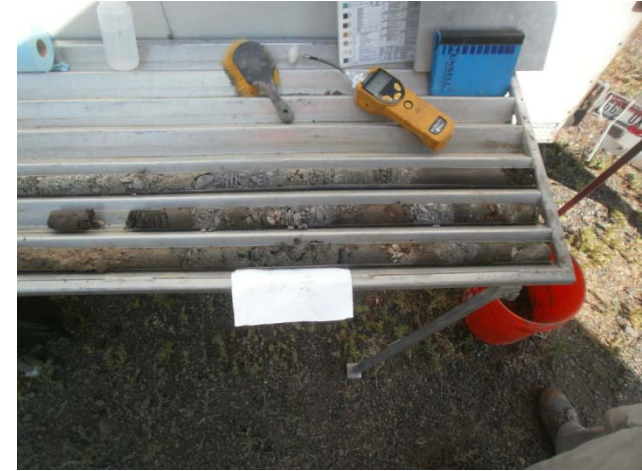
Soil core from boring BH-18.
