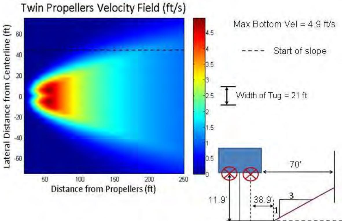
**Figure 4. Whatcom Waterway near-bottom propwash velocity, Run 3**
