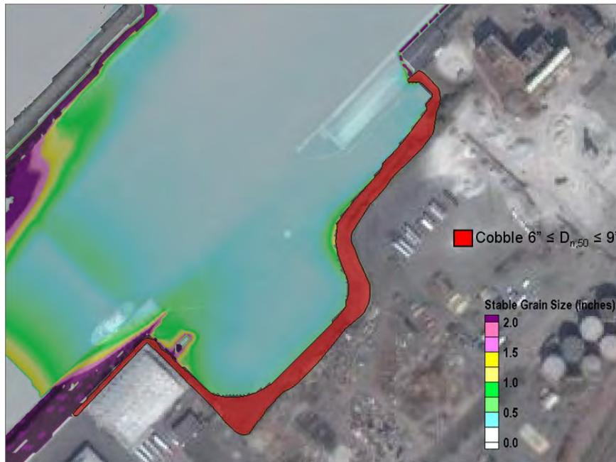
**Figure 5. Stable material size according to location, wave direction from 240 degrees**
