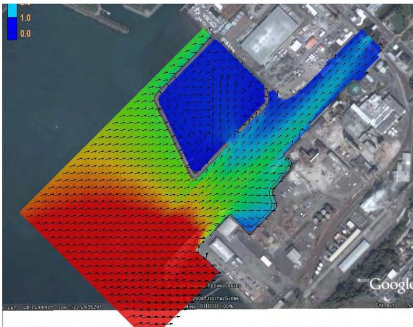
**Figure 4. Wave height and direction in Whatcom Waterway, wave storm approaching from 270 degrees**
