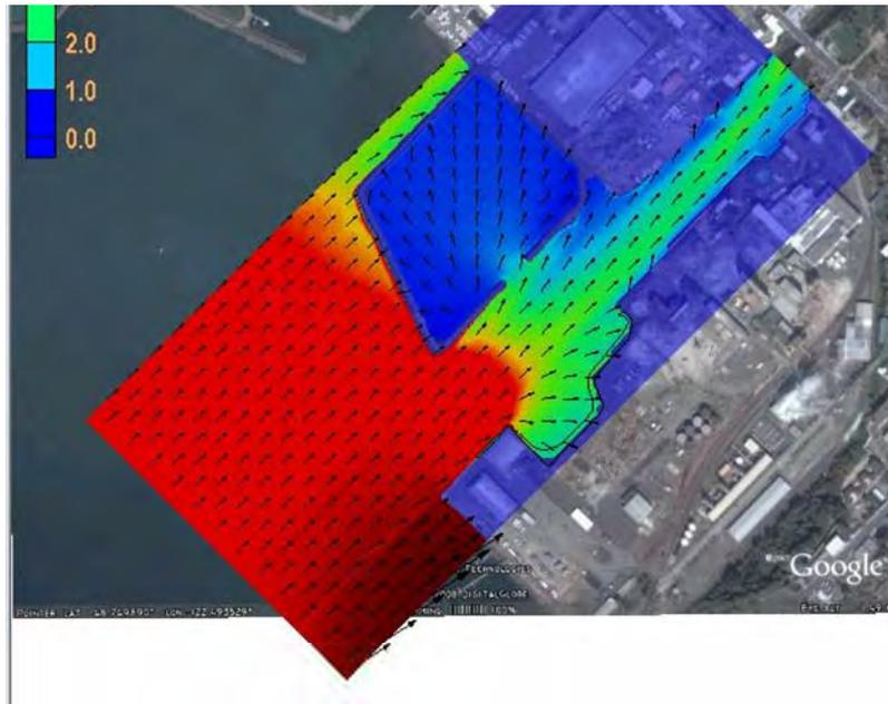
**Figure 3. Wave height and direction in Whatcom Waterway, wave storm approaching from 240 degrees**
