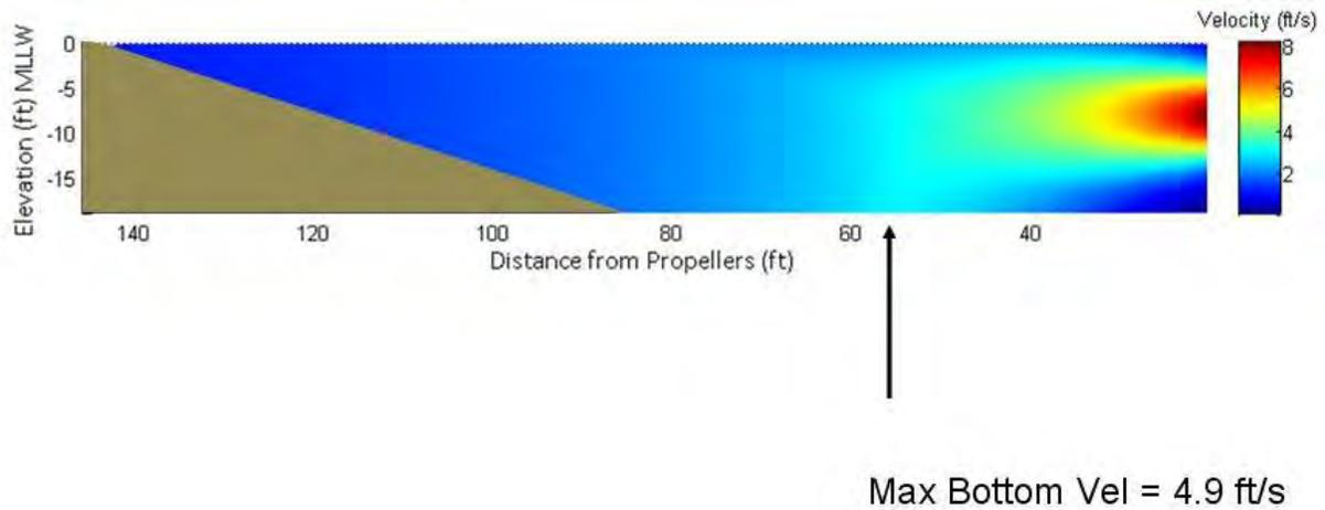
**Figure 8. Whatcom Waterway vertical slice through axis of propwash velocity, Run 6**
