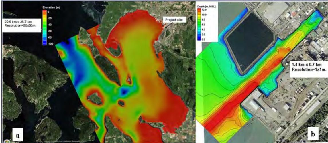
Figure 1. Large (a) and nested (b) wave numerical modeling domains
