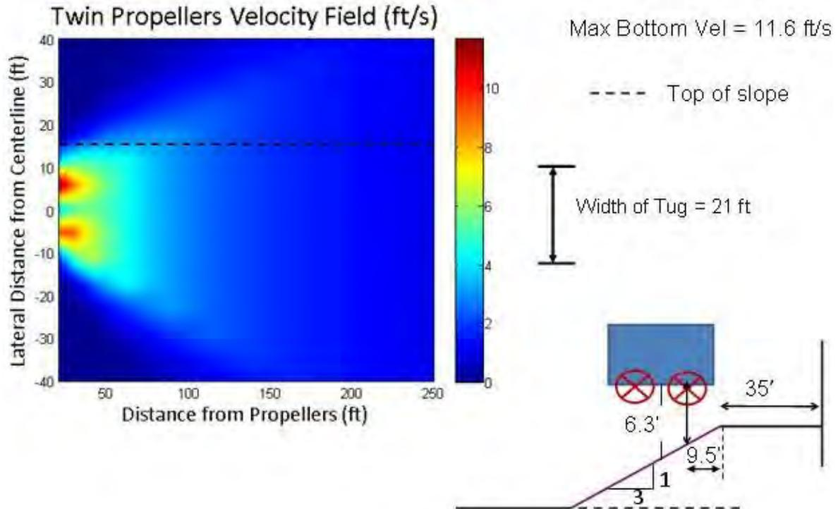
**Figure 5. Whatcom Waterway near-bottom propwash velocity, Run 4**
