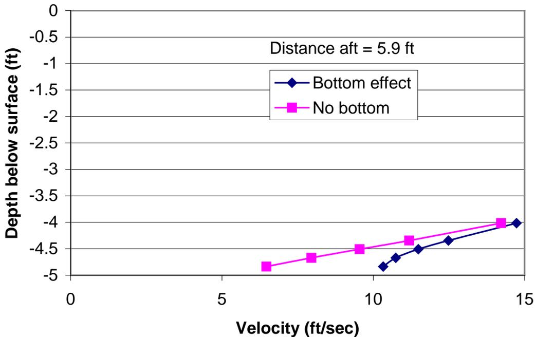
Figure 4. Example of JETWASH computational test, Monterey boat in 5-ft depth
