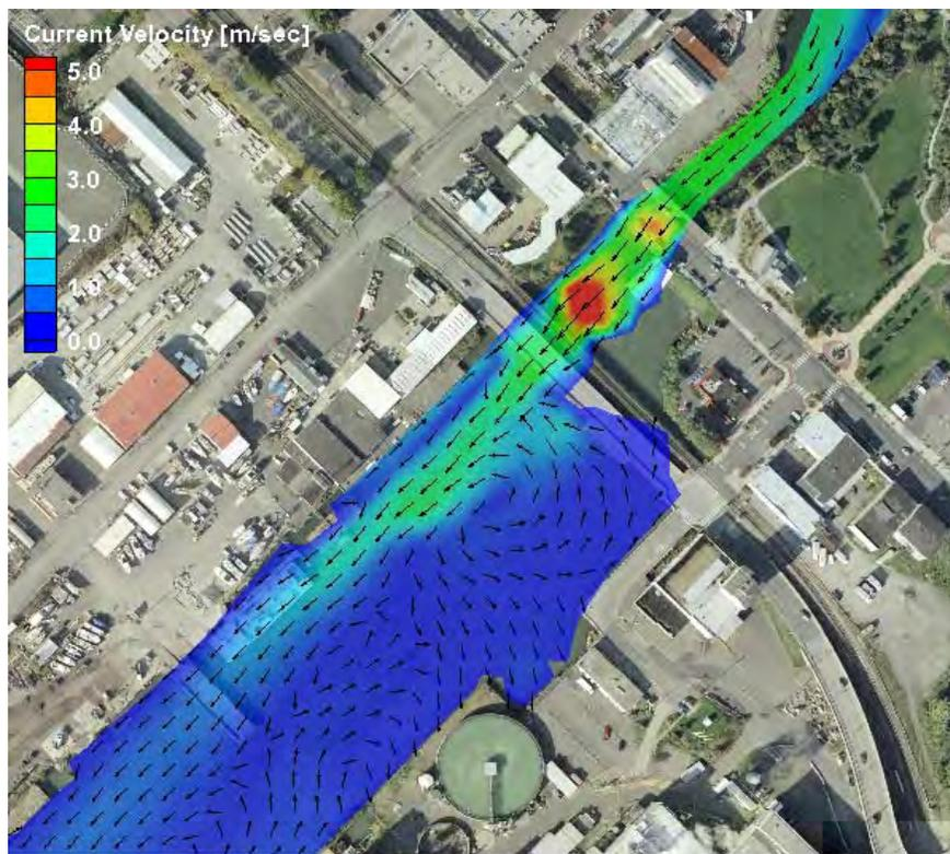
Figure 8. Velocity pattern at time of peak flow, depth-averaged velocity
