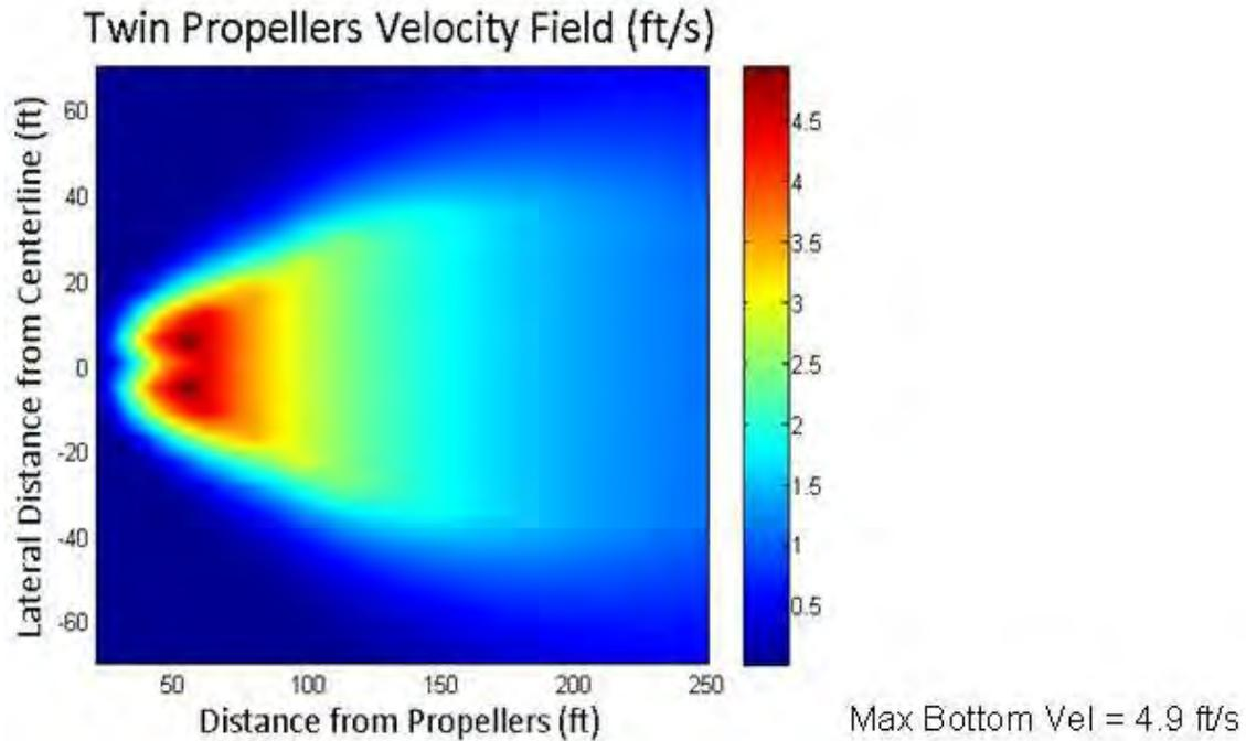
**Figure 7. Whatcom Waterway near-bottom propwash velocity, Run 6**
