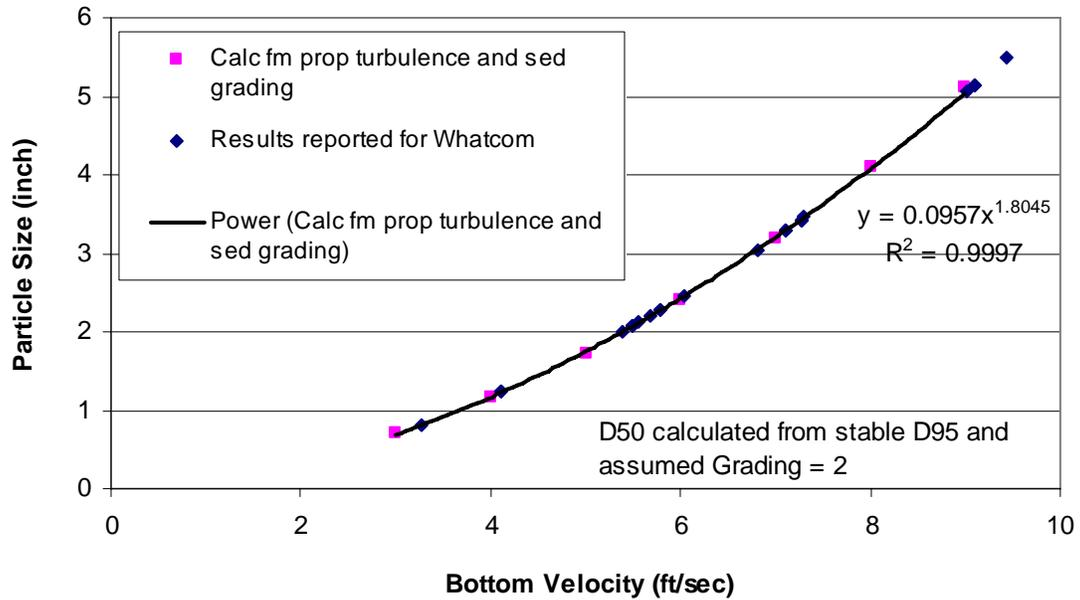
Figure 11. Near-bottom velocity and corresponding stable particle size
