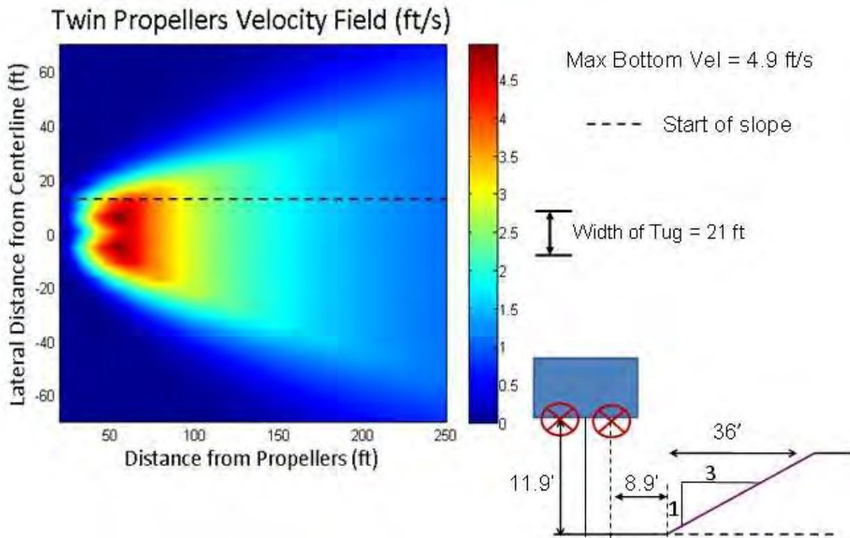
**Figure 6. Whatcom Waterway near-bottom propwash velocity, Run 5**
