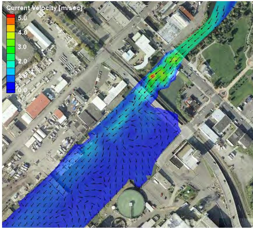
**Figure 9. Velocity pattern at time of peak flow, bottom velocity**
