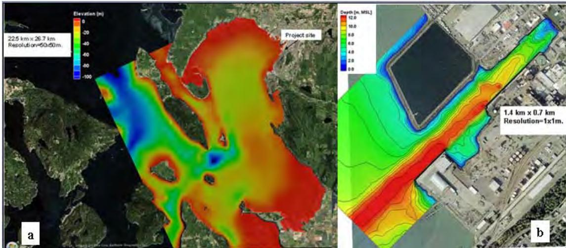
Figure 1. Large (a) and nested (b) wave numerical modeling domains
