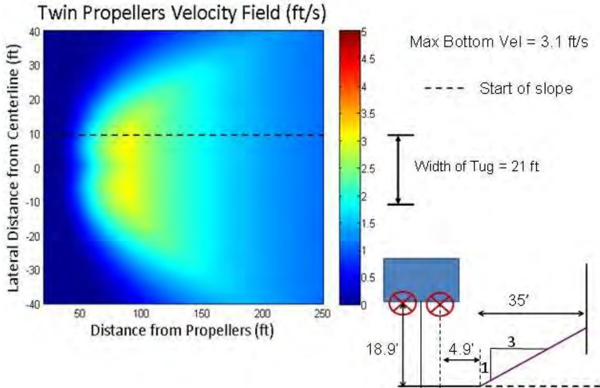
**Figure 3. Whatcom Waterway near-bottom propwash velocity, Run 2**
