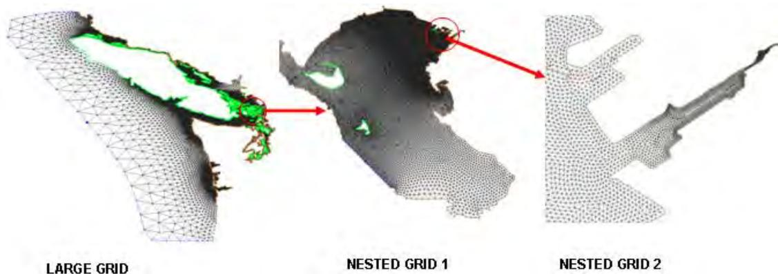
**Figure 6. SELFE numerical modeling grids for Whatcom Waterway hydrodynamic modeling**
