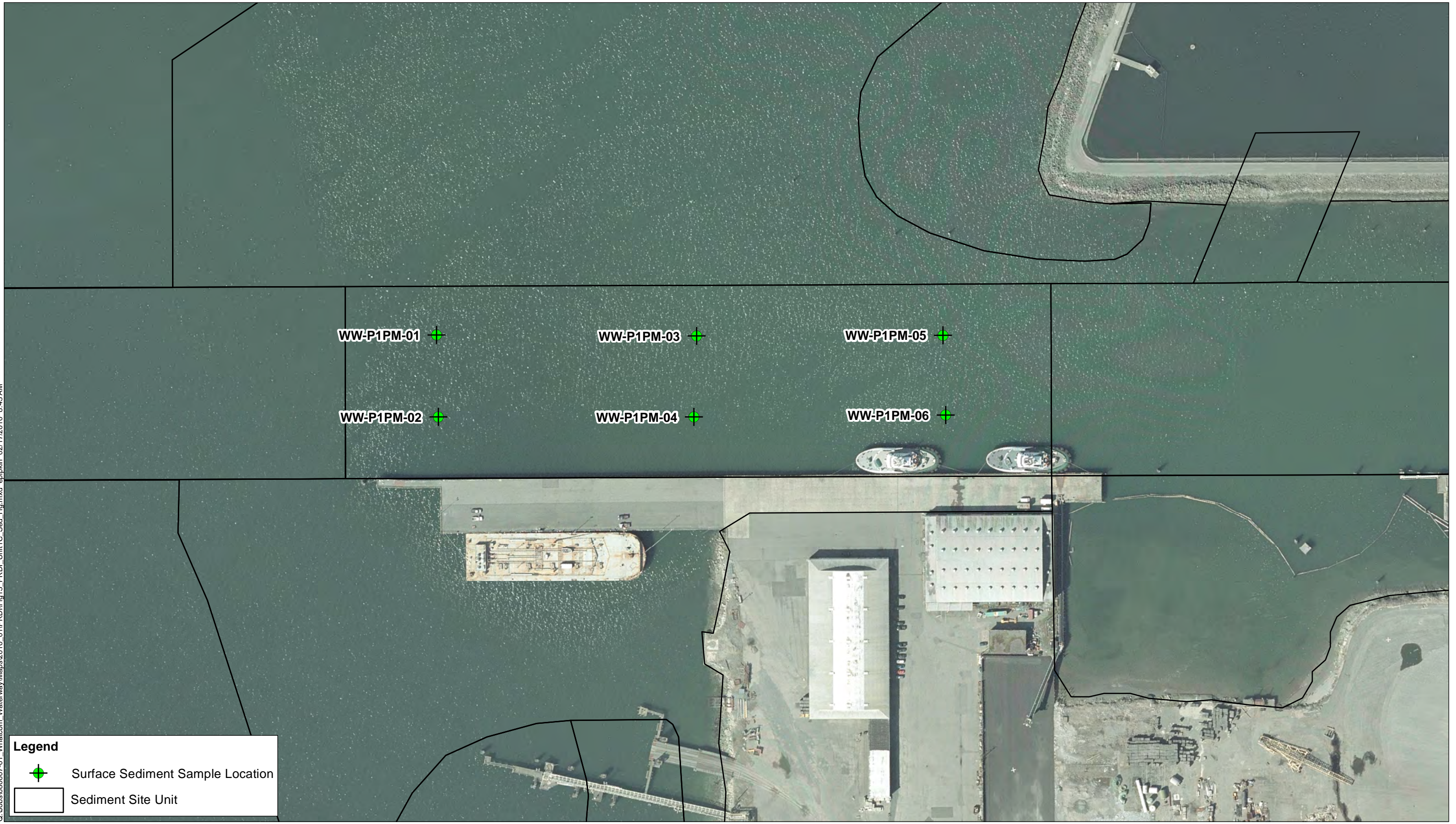
Figure 2 Performance Monitoring Surface Sediment Sampling Locations Appendix G - Compliance Monitoring and Contingency Response Plan Whatcom Waterway Cleanup in Phase 1 Site Areas - Final EDR
