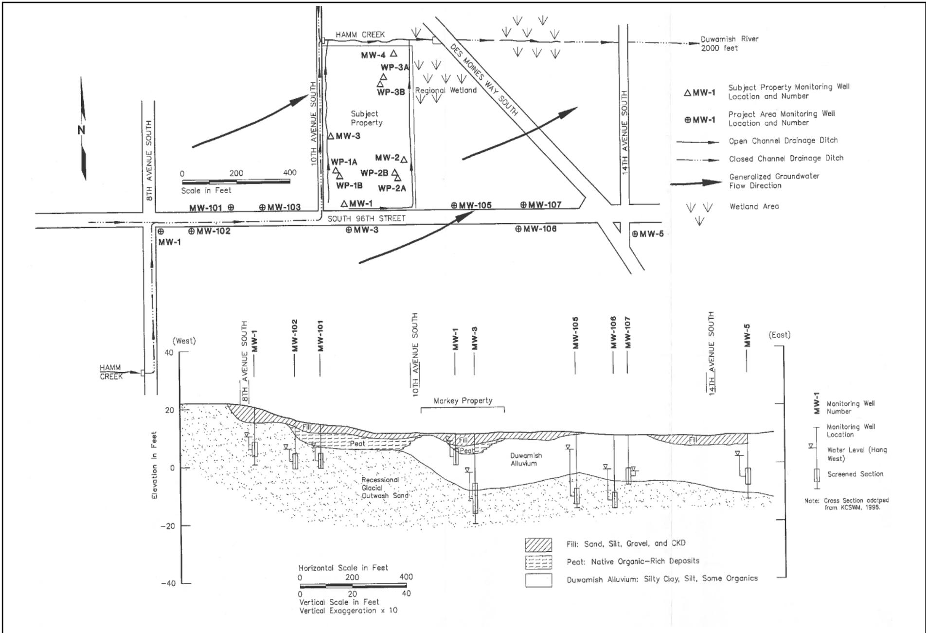
Figure 14. Hydrogeologic Cross-Section of S 96th Street
