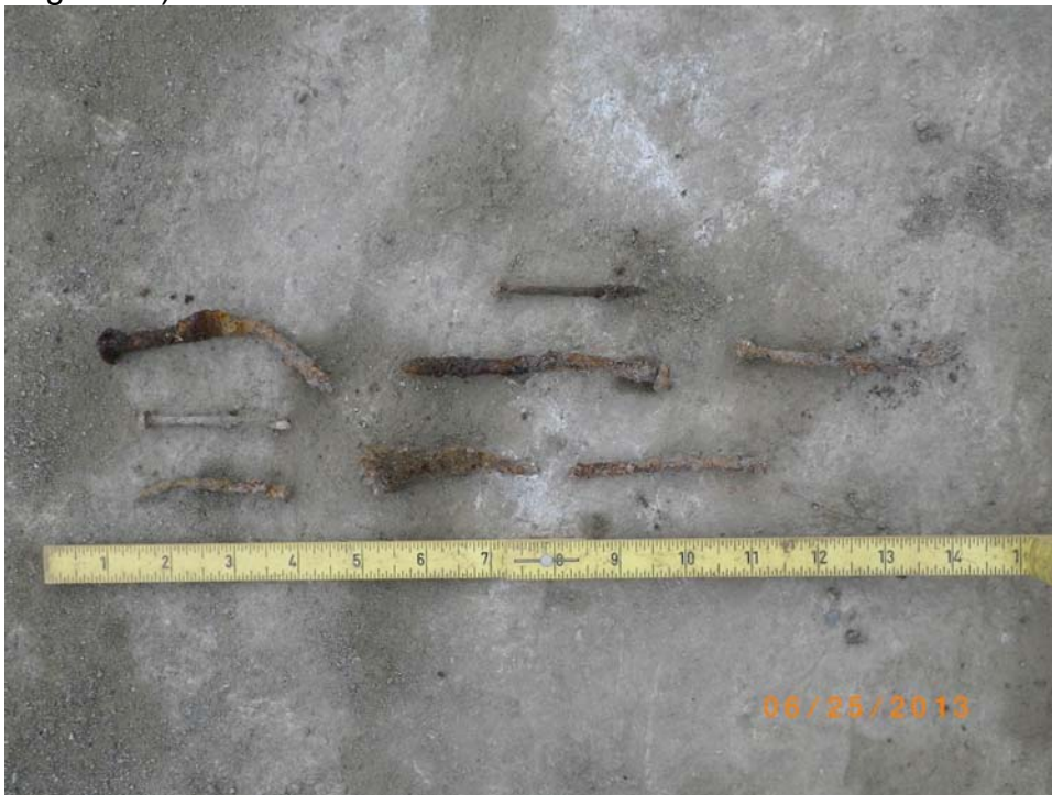
Photograph 10. Assorted wire nails observed within rubble and fill.
