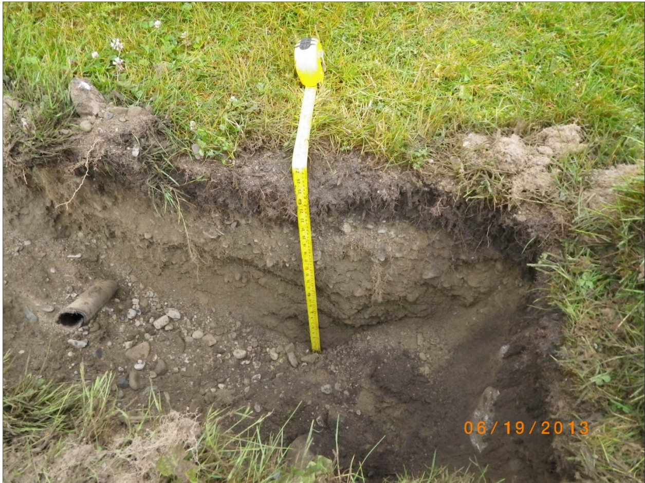
Figure 5-2. View to west of the fill and overburden sediments exposed in Sample S35-G-11 (0 to 27 inches below surface). Note gravelly and cobbly fill and truncated utility pipe.
