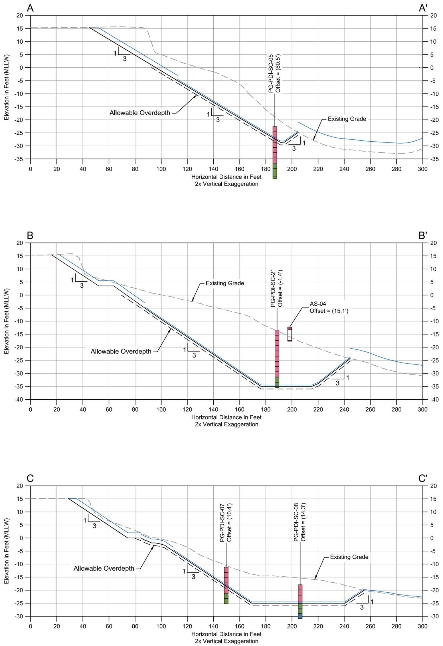
**SURVEY:** Bathymetry from Triad Associates, dated 2012, and eTrac, dated August 27, 2014.
