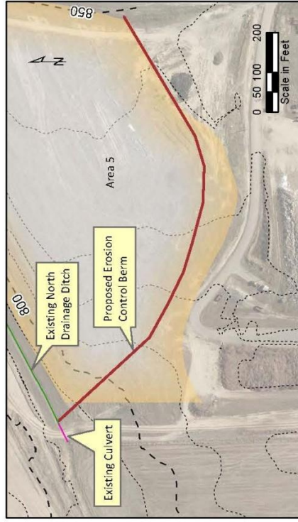
Plate 3: Area 5 Erosion Control Berm--Plan View
