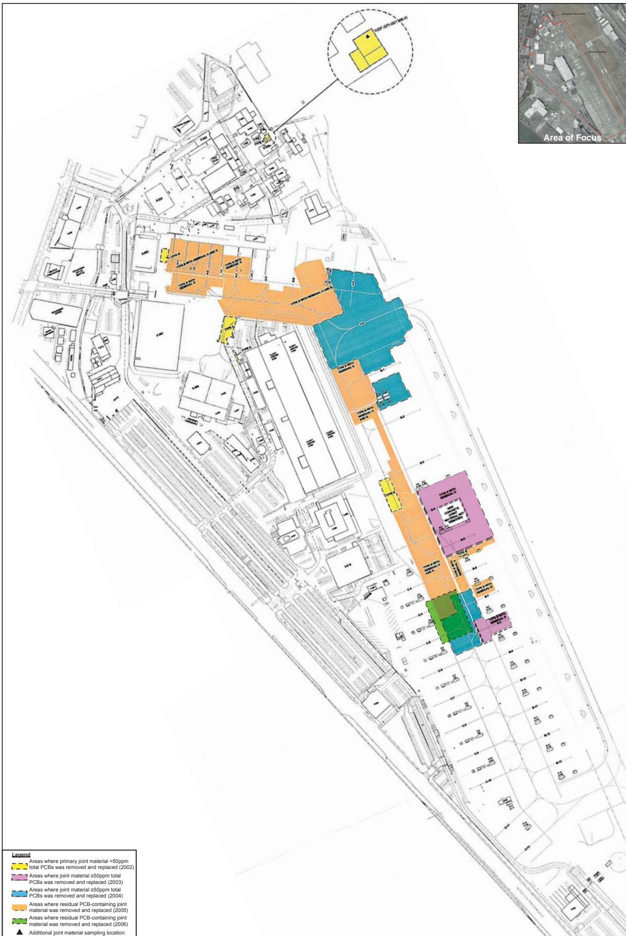
Figure 4-44. Concrete Joint Material Removal Areas (2002 - 2006)
