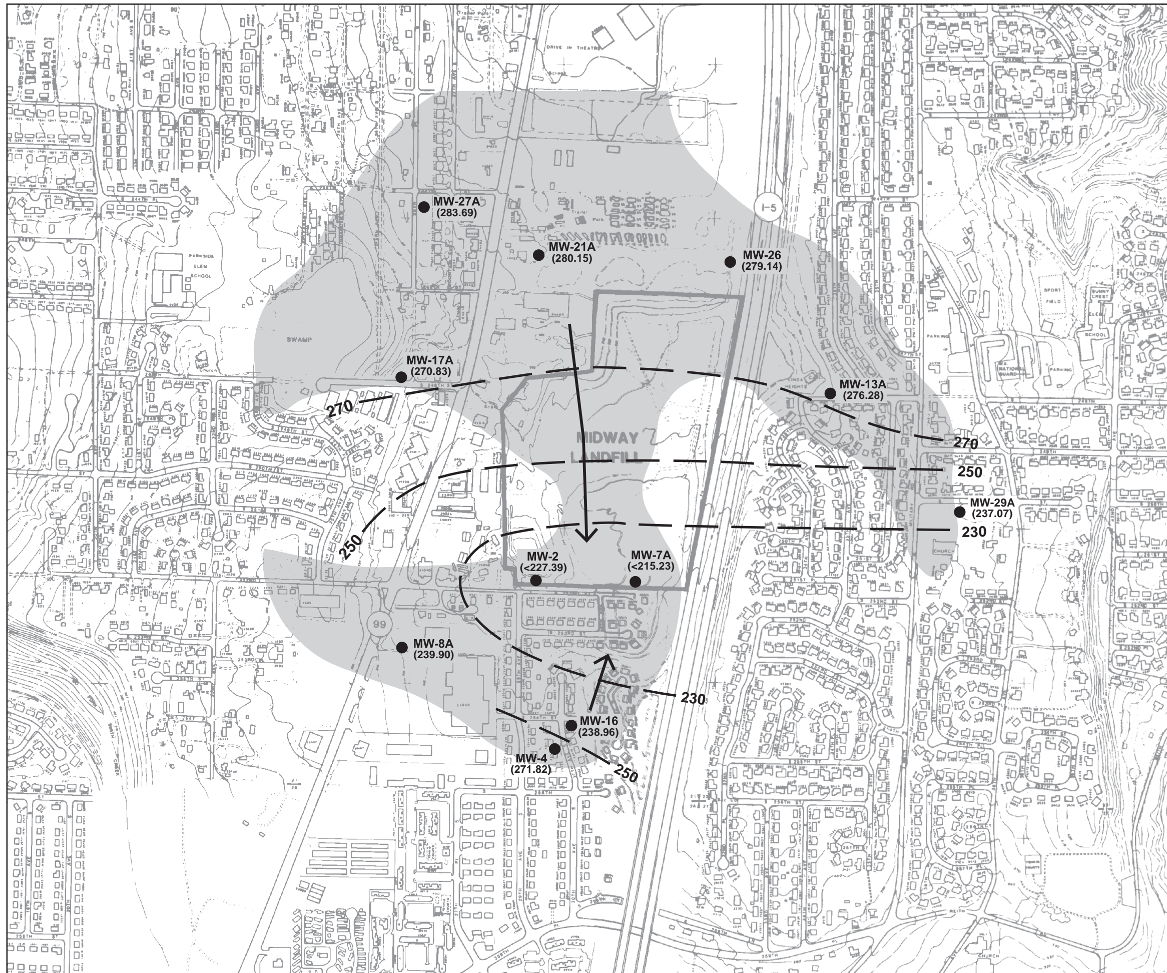
Figure 2-11 Generalized Upper Gravel Aquifer Potentiometric Surface Map, May 2014 Midway Landfill Kent, Washington
