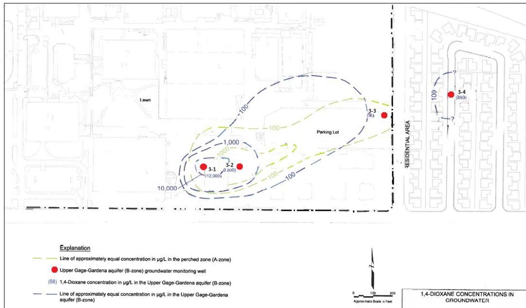
Figure 4. Site 3 map. Monitoring wells marked as red dots, dioxane concentrations marked as dashed green or blue lines.
