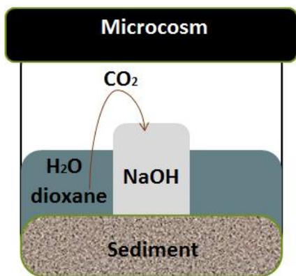
Figure 6. Diagram of new microcosm design.
