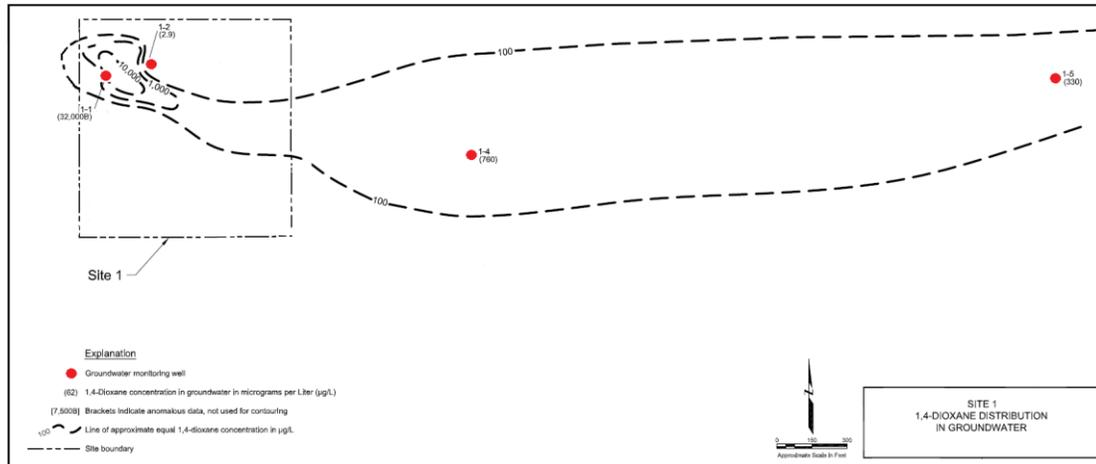
Figure 3. Site 1 map. Monitoring wells marked by red dots, dioxane contour lines marked as black dashed line.
