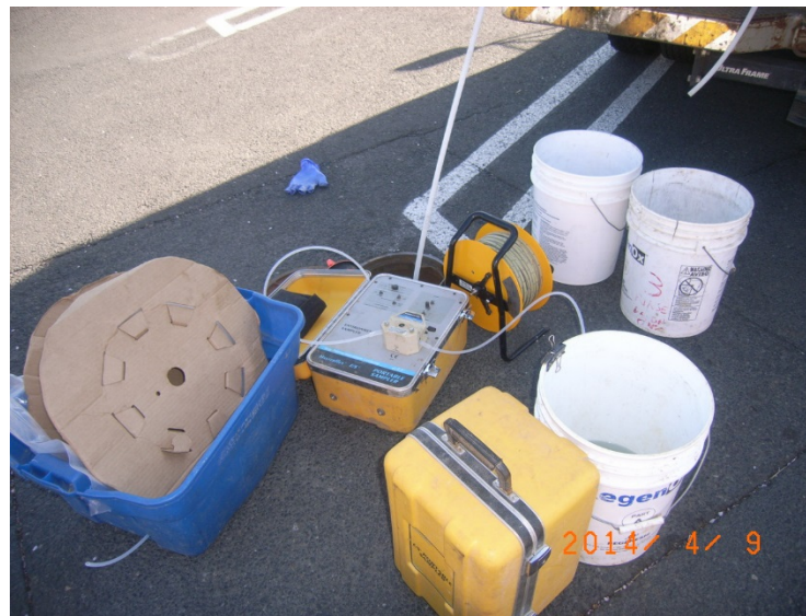
Purging ground water from monitoring well KMW-04.
