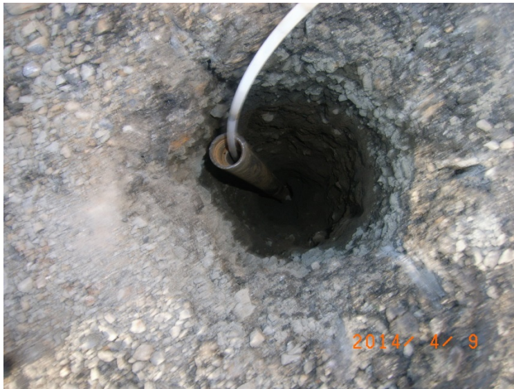
View down hole in EB1A showing the gravelly character of the soil.
