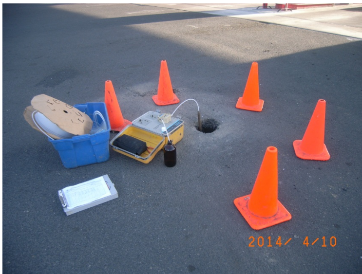
Sampling ground water at EB1A – view northeast.
