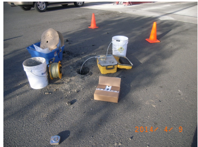
Purging ground water from EB1A – view northeast.
