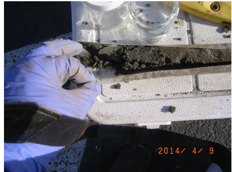
Close-up showing recovered saturated soil from EB1A.
