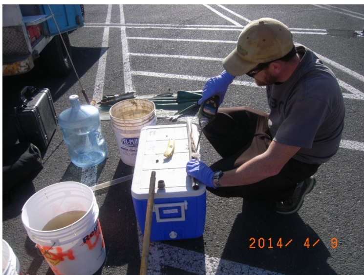
Retrieving soil core from manual DPT sample sleeve and screening with a PID.
