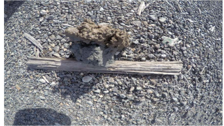
Sharp contact between stained silt and overlying un-impacted silty sand at TP-10.
