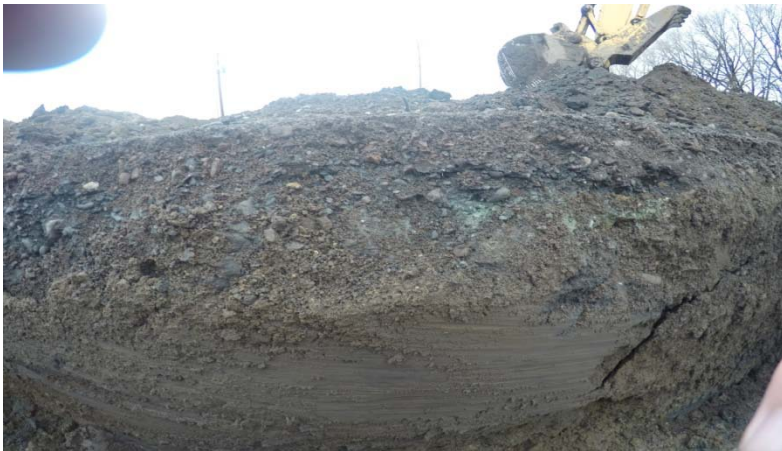
This is a photo of a surface trench. Variable soil coloration can be seen indicating possible, but minimal contamination.
