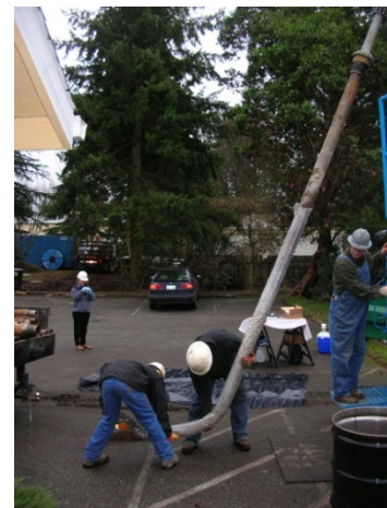
Photograph 12. Sample collection from a SONIC drill rig on the TOC/Farmasonis Property.
