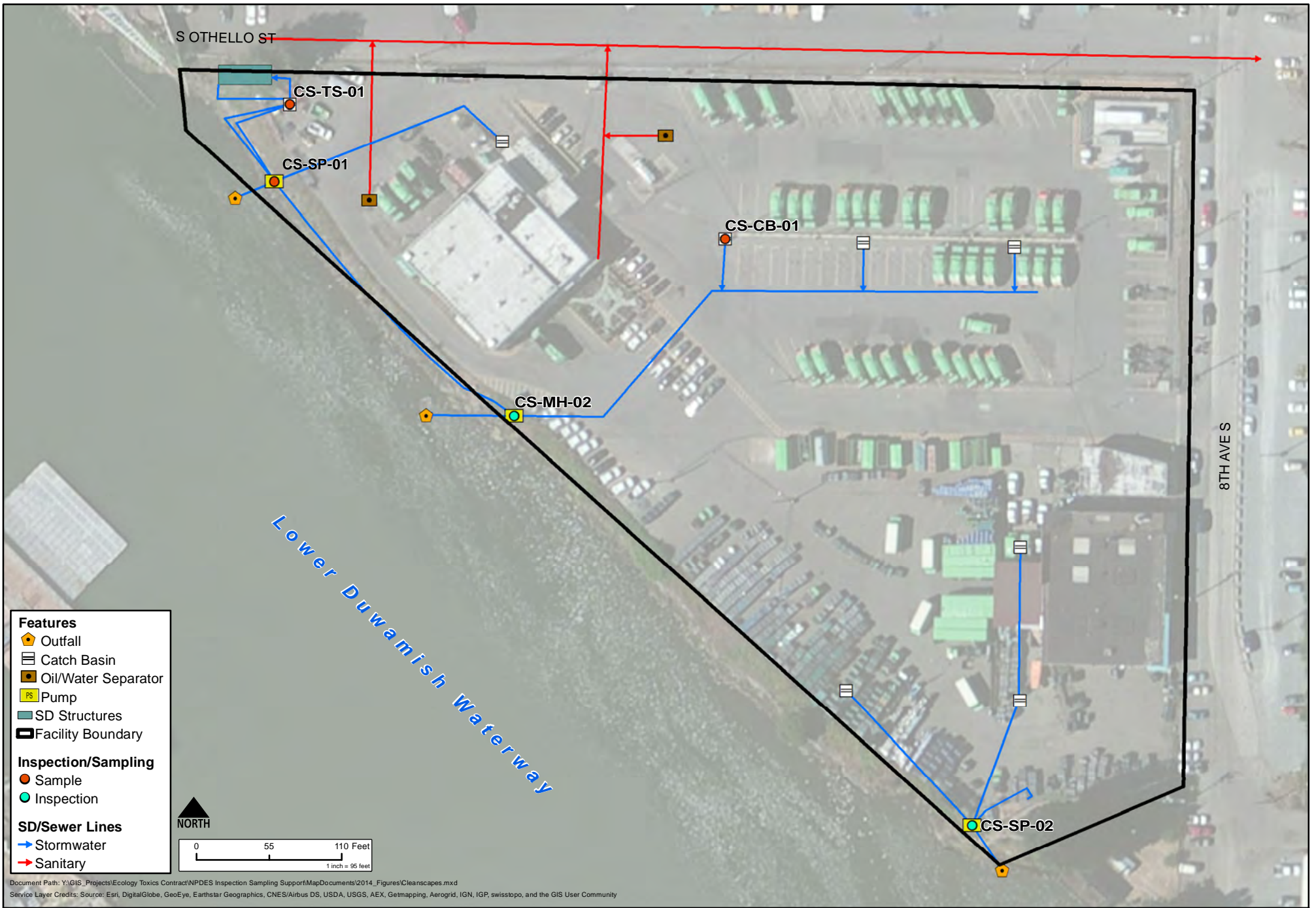
Figure L-2. Recology CleanScapes Inspection and Sample Locations
