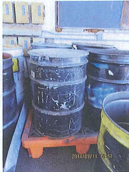
#10. DESCRIPTION: Drums stored on spill pallets.
