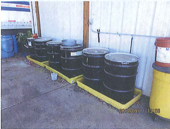
#9. DESCRIPTION: Drums stored in secondary containment trays.
