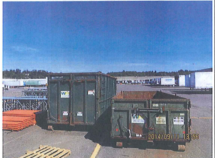
#4. DESCRIPTION: Scrap-metal dumpsters left uncovered when not engaged in active filling/unloading.
