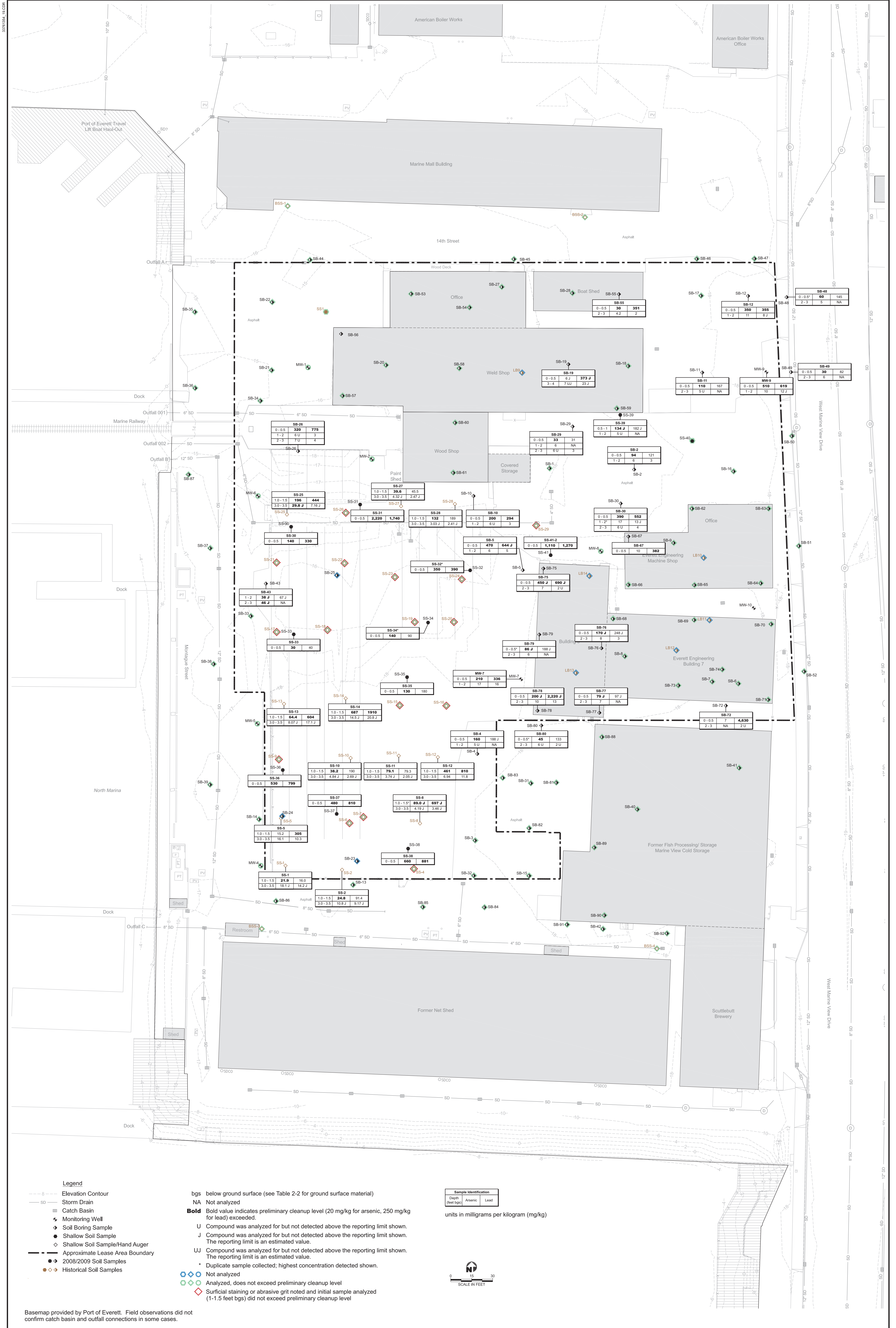
Figure 4-1 Extent of Arsenic and Lead Impacted Soil
