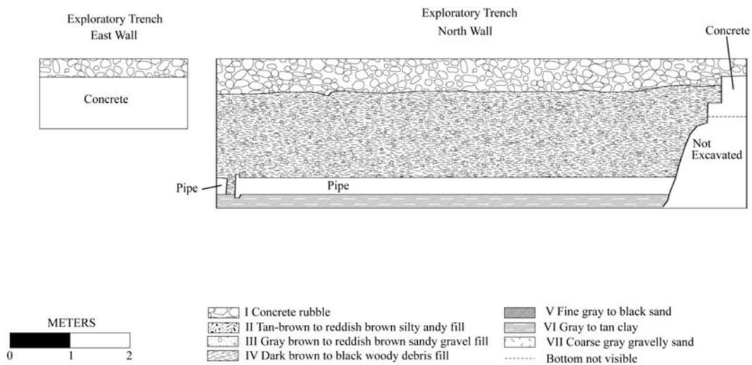
**Figure B5.** Profile of exploratory trench (see Figure B1).
