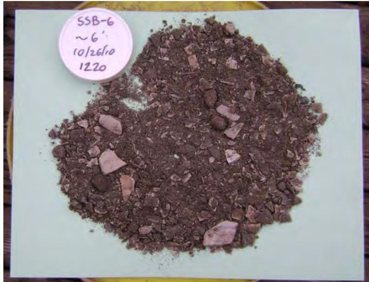
Figure 10. Fragmented shell and sand from SSB-6, about 6 ft. below surface.
