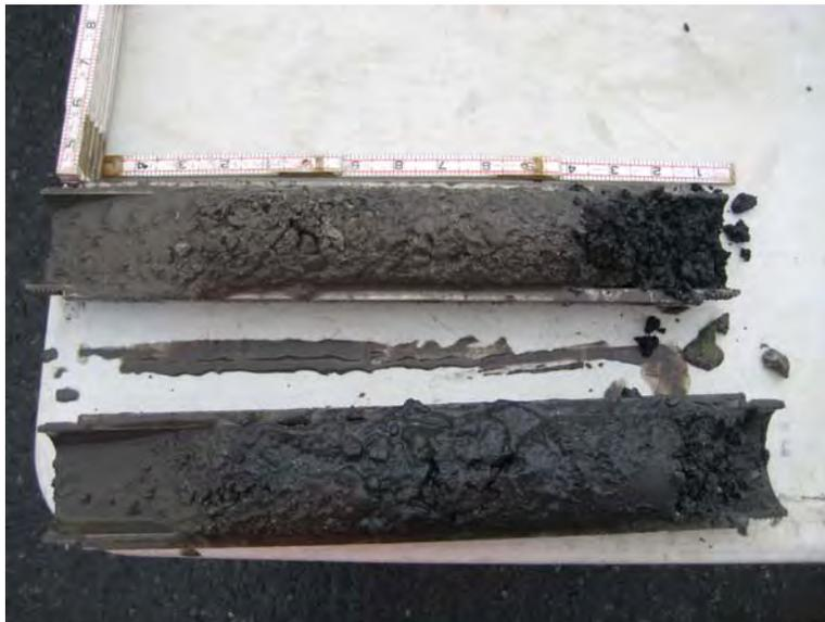
Figure 16. MW-68 core with beach sediments.
