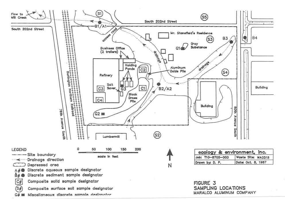
All samples collected were analyzed for total priority pollutant metals. The solid, soil and sediment samples were also analyzed for leachable metals in accordance with the EP Tox procedure (12).
