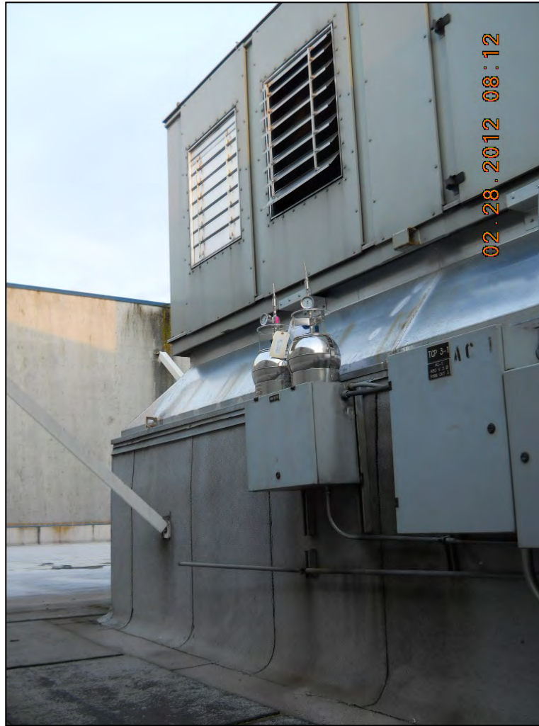
1. Ambient air sample AA01 at Fana West. Two canisters set due to initial concern about flow controller of first can.
