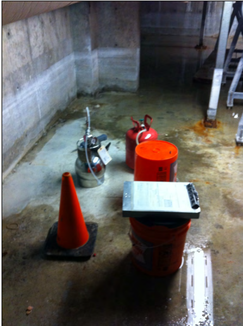
15. Sub-slab soil vapor (i.e. soil gas) sample SSV46 at YMCA collected in crawl space beneath pool.
