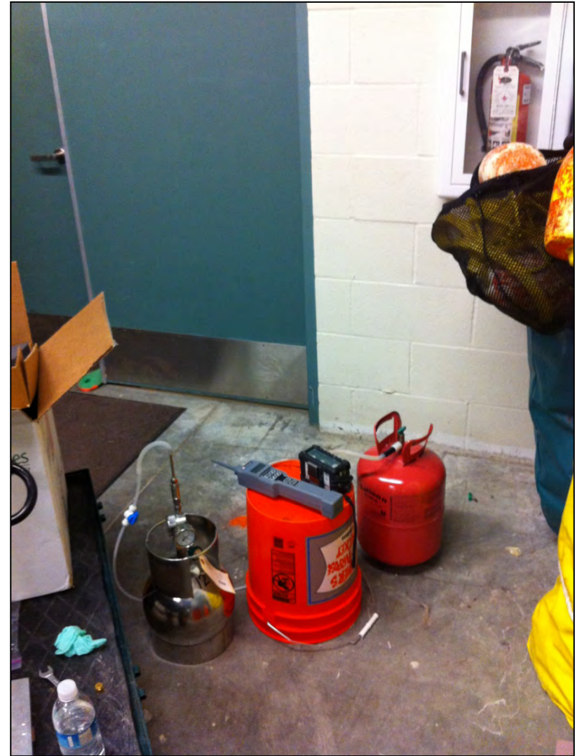
16. Sub-slab soil vapor (i.e. soil gas) sample SSV47 YMCA collected in boiler room.
