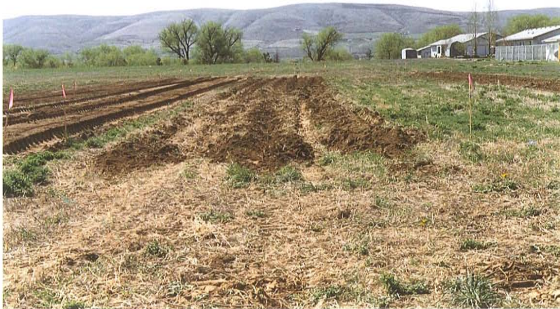
Figure 1: View of N - S test plots following soil ripping (center) and road reclaiming (far left)
