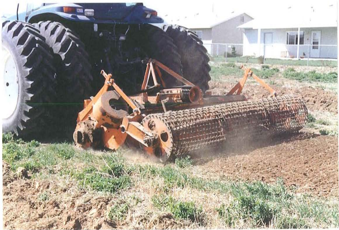
Figure 8: Roto-tiller at N - S test plot: steel mesh in back of tiller acts to smooth soil.
