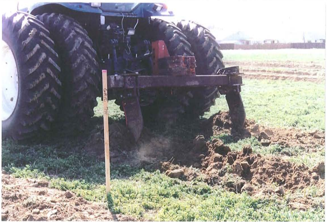
Figure 7: Soil ripping prior to roto-tilling.
