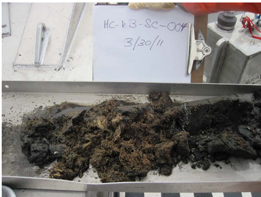
Photograph 11 - Example of wood debris found in a vibracore tube sample. Note the smaller wood fibers seen in this sample.
