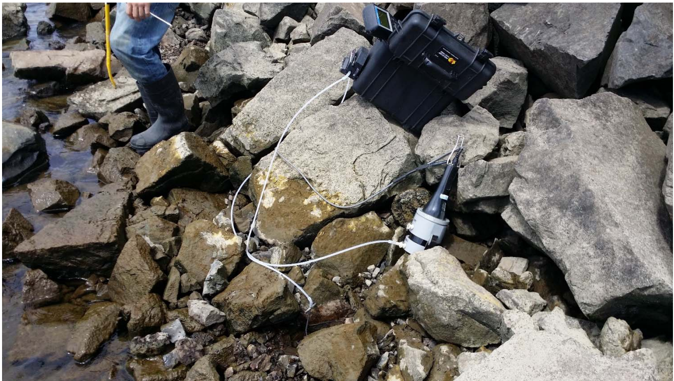
Photograph 4: Typical pore water sampling setup.
