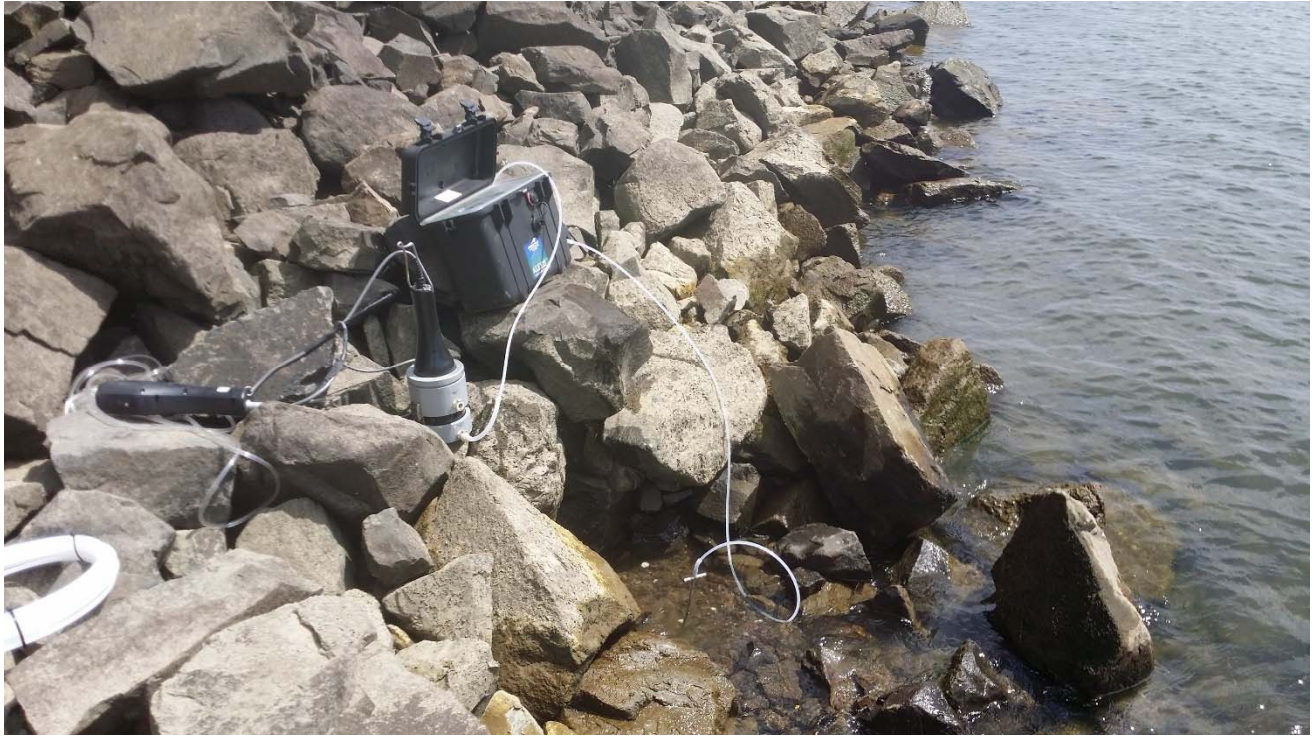
Photograph 3: Typical pore water sampling setup.
