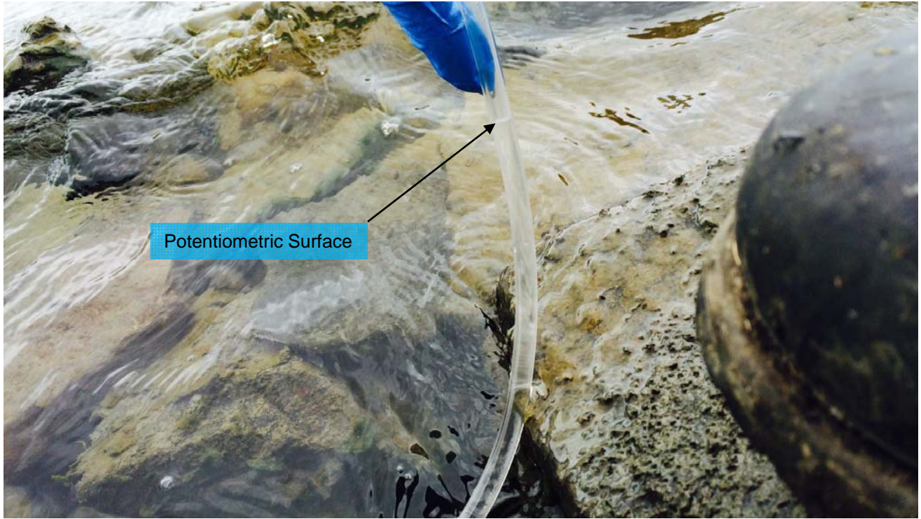
Photograph 5: Pore water potentiometric surface relative to river surface.
