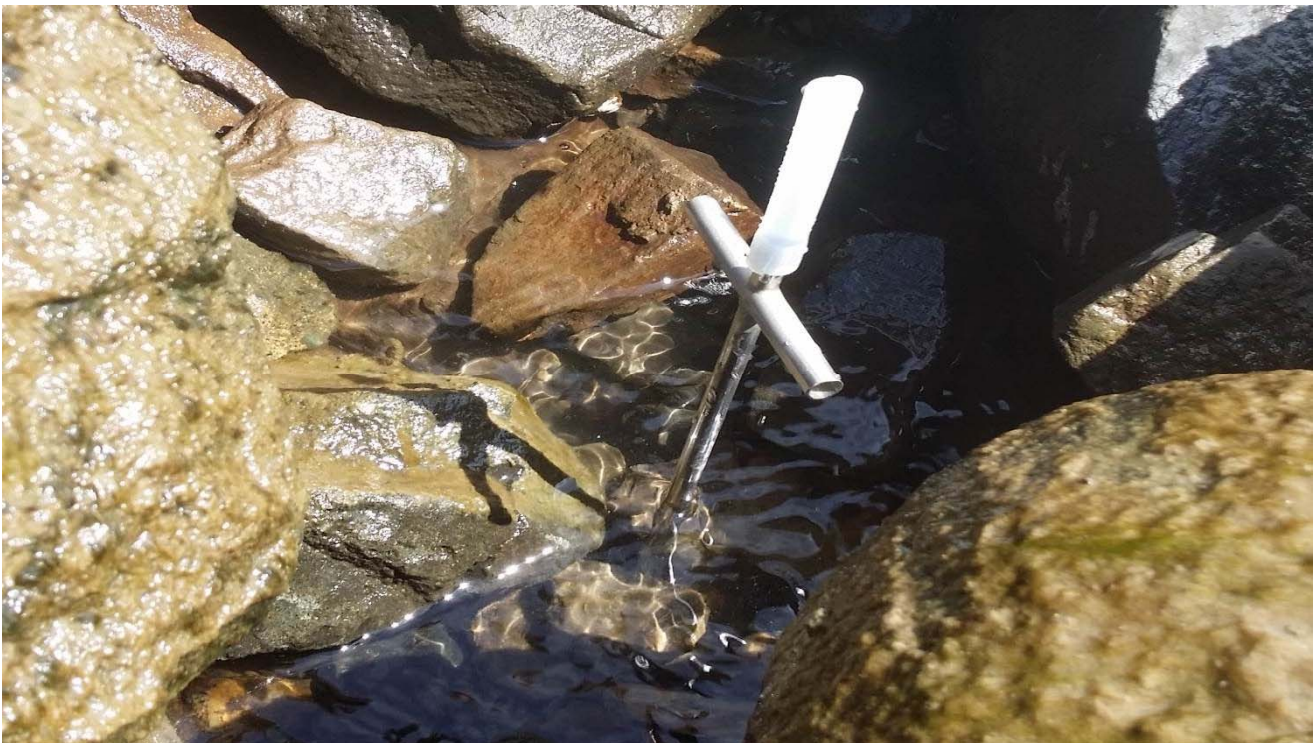
Photograph 6: Artesian flow from Pushpoint sampler.
