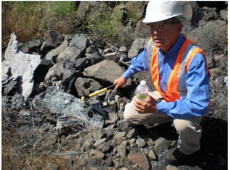
Figure 3 – Bill Bath Using Hammer Test on Tentatively Identified Spent Potliner at Goldendale – July 2010.
