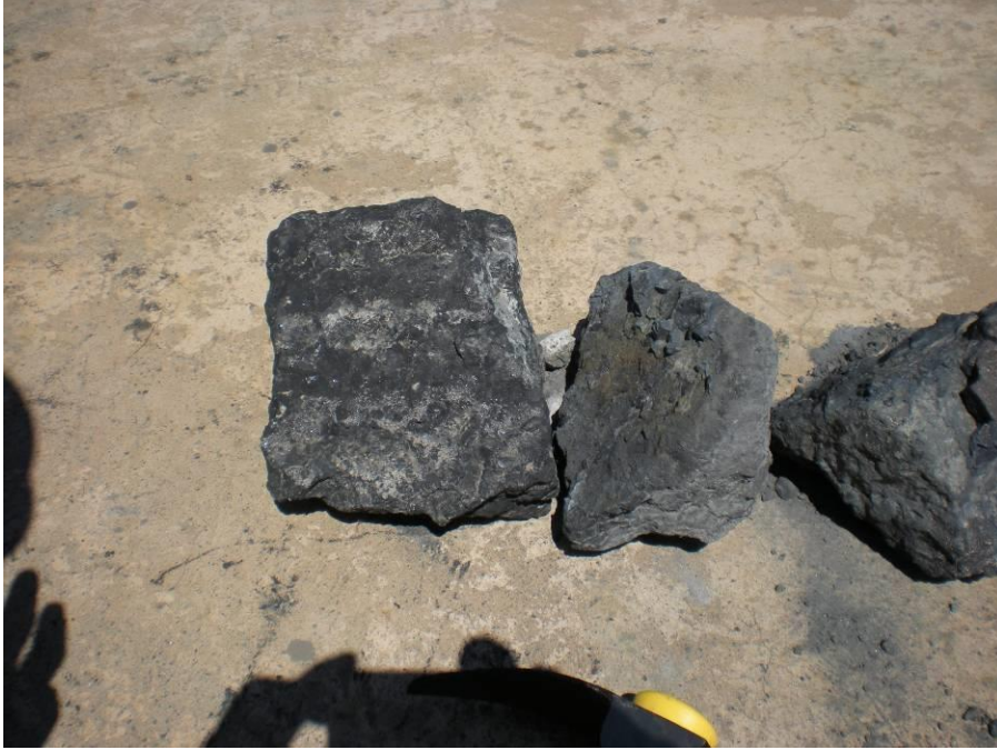
Figure 2 – Tentatively Identified Spent Potliner Examples Discovered at “Smelter Sign Area” – July 2010.
