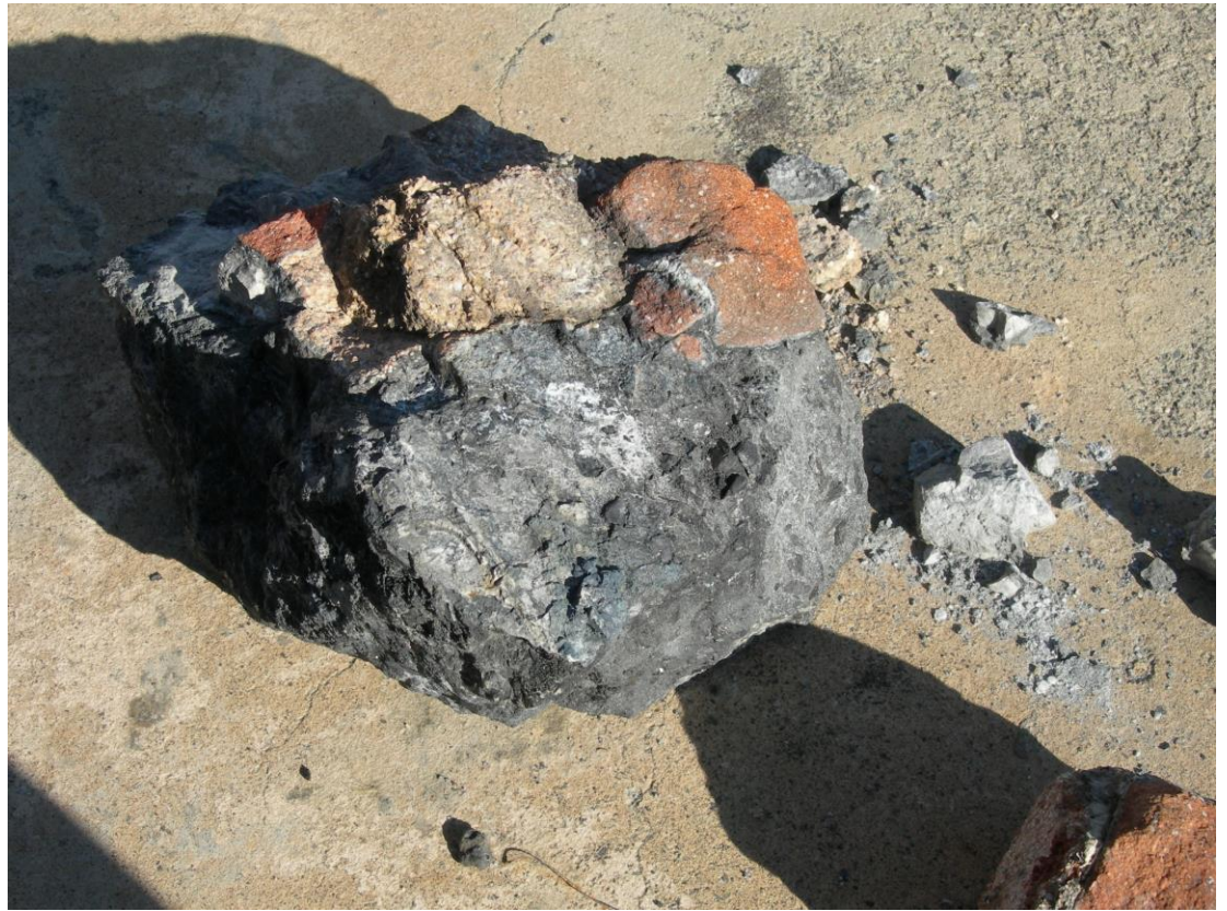
Figure 6 – SPL showing white salt deposits, gray-blue cast and recrystallization
