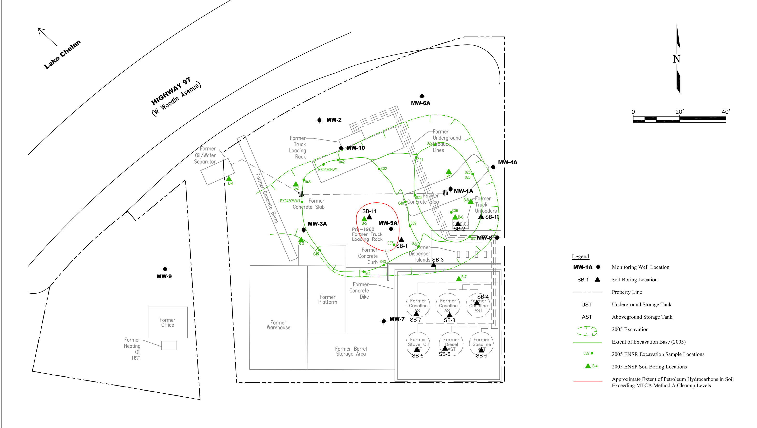
FIGURE 2 Extent of the 2005 Excavation and Extent of Petroleum Hydrocarbons in Soil
