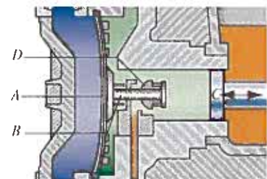
Figure 3 Diaphragm (A) and piston (C) are full rearward, once again forcing Mars valve (B) to its rearward position, which allows poppet (D) to open if required. Low oil volume creates a vacuum and opens poppet, permitting hydraulic fluid to enter the chamber from the refill line.
