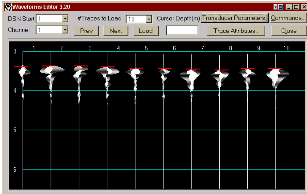
Figure 6: High quality FWF data. The bottom pick is indicated by the horizontal red line.
