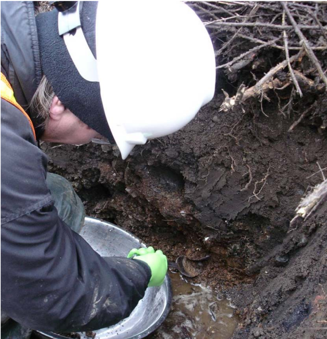
TP-22 Sampling at 1.7-2.2 ft bgs
