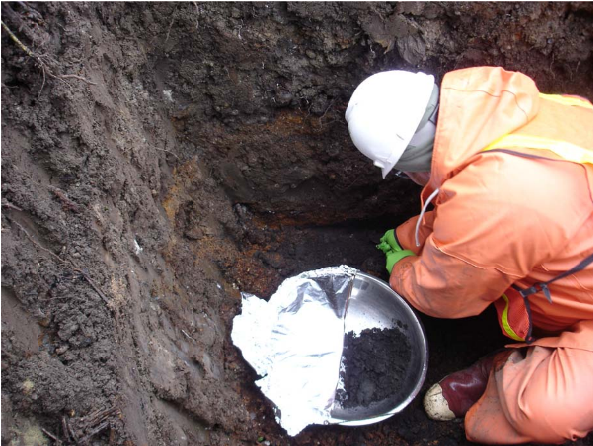
TP-23 Sampling at 4 ft bgs
