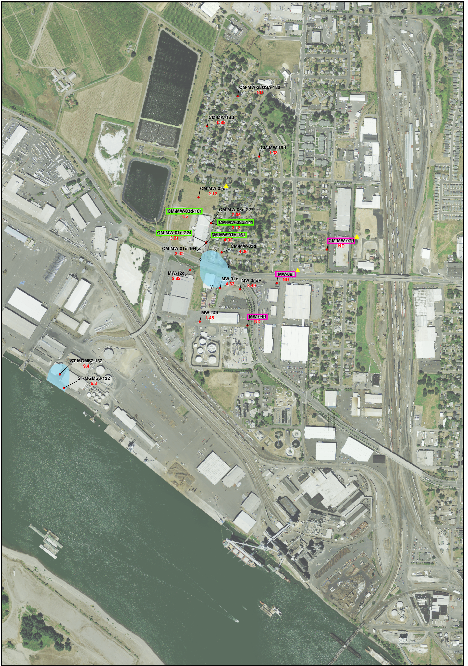
Figure 6 PCE Isoconcentrations in Deep USA Zone Groundwater 1st Quarter 2015
