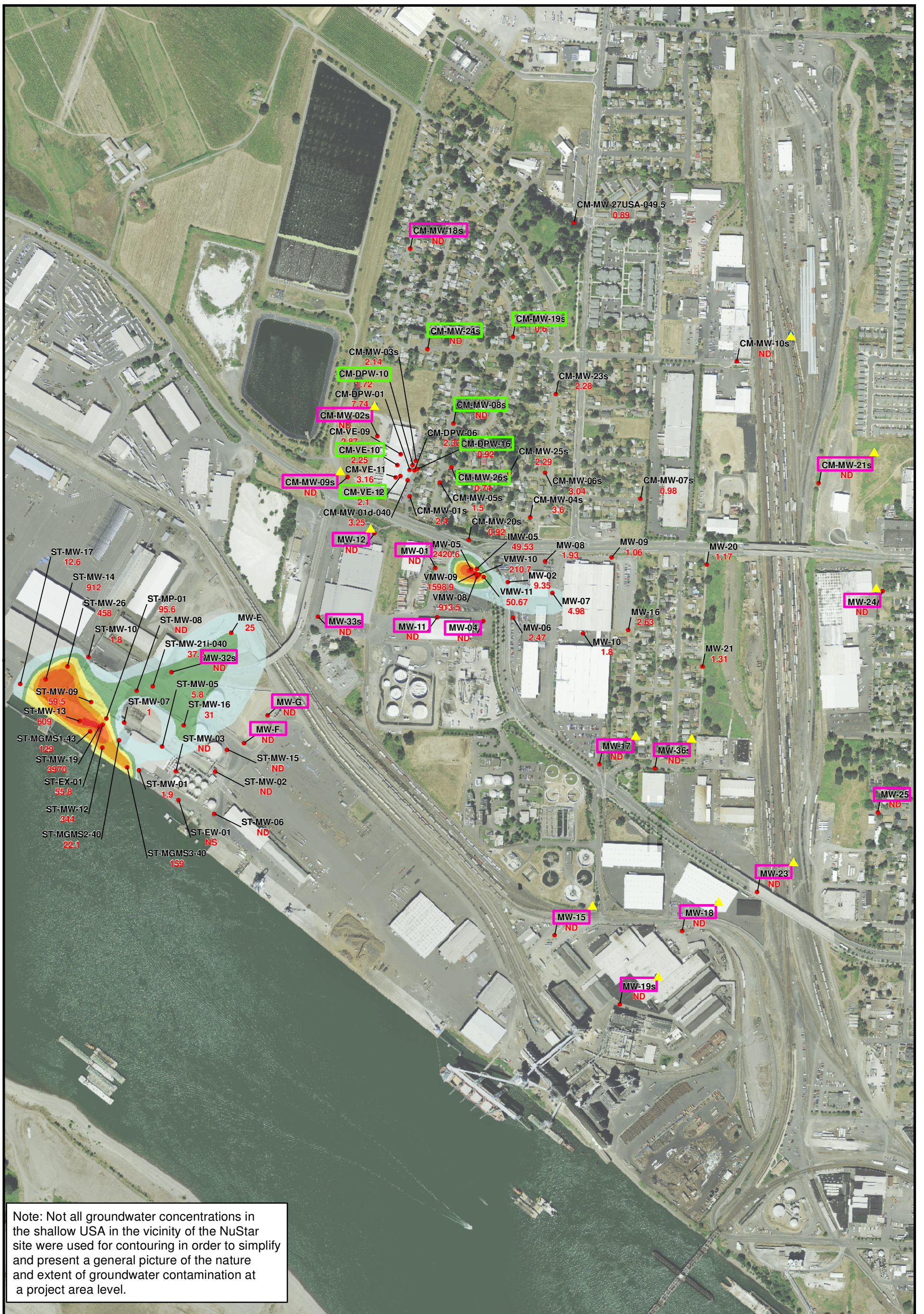
Figure 1 TCE Isoconcentrations in Shallow USA Zone Groundwater 1st Quarter 2015
