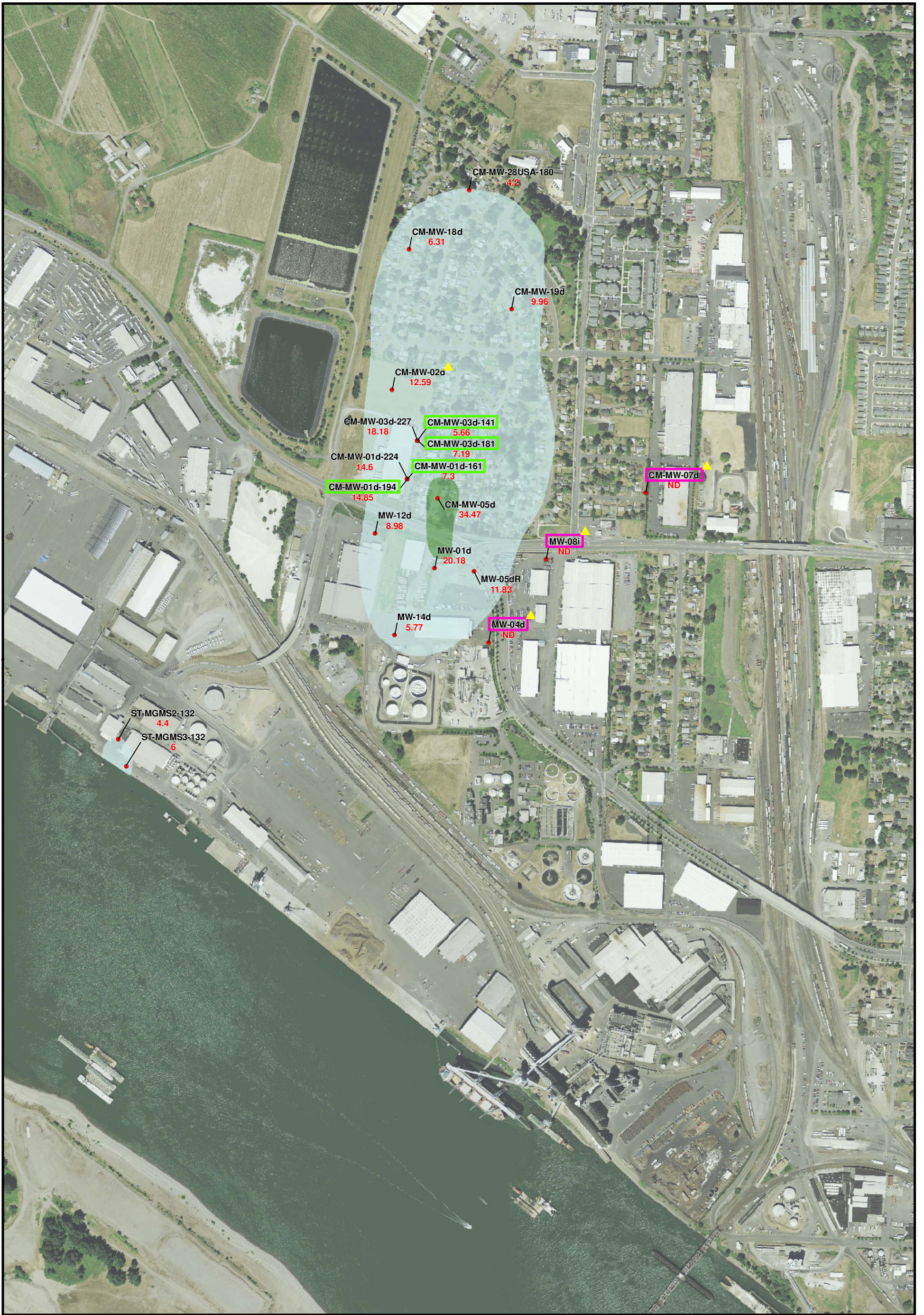
Figure 5 TCE Isoconcentrations in Deep USA Zone Groundwater 1st Quarter 2015
