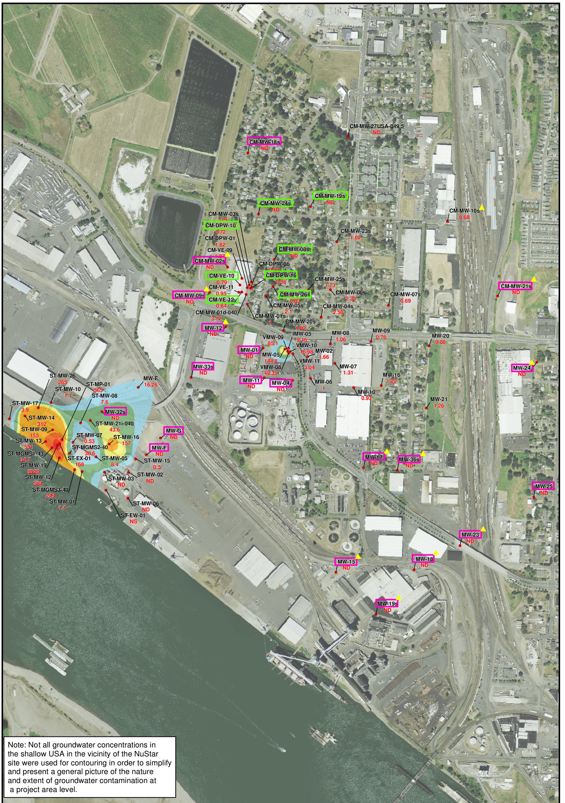
Figure 2 PCE Isoconcentrations in Shallow USA Zone Groundwater 1st Quarter 2015
