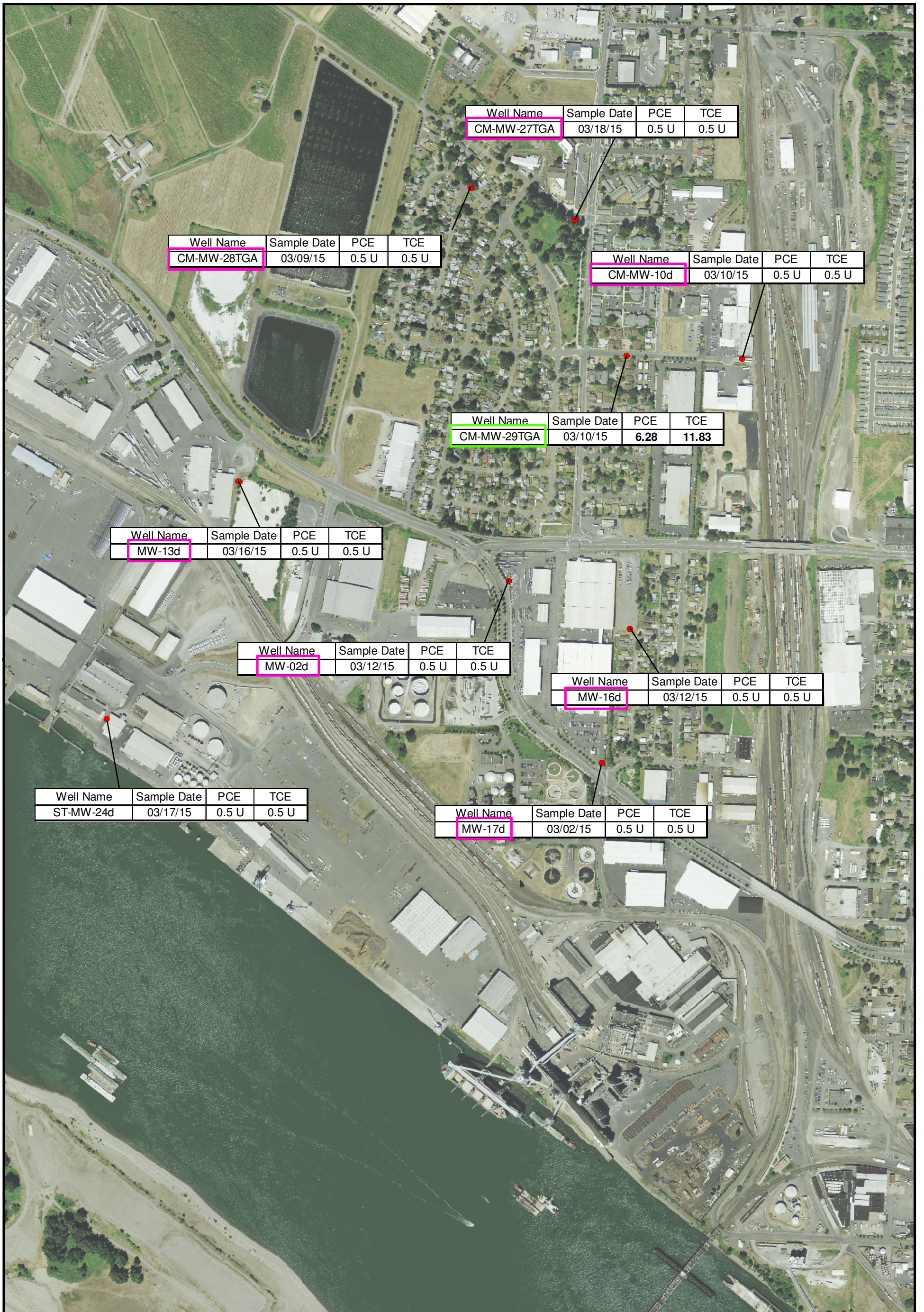
Figure 7 2015 TCE and PCE Concentrations in the TGA
