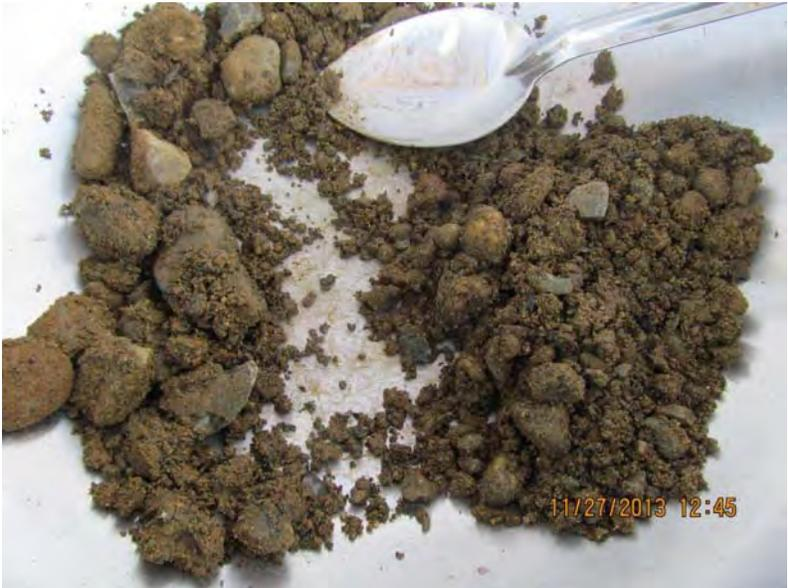
Photo 11. Sample obtained from crib wall core.
