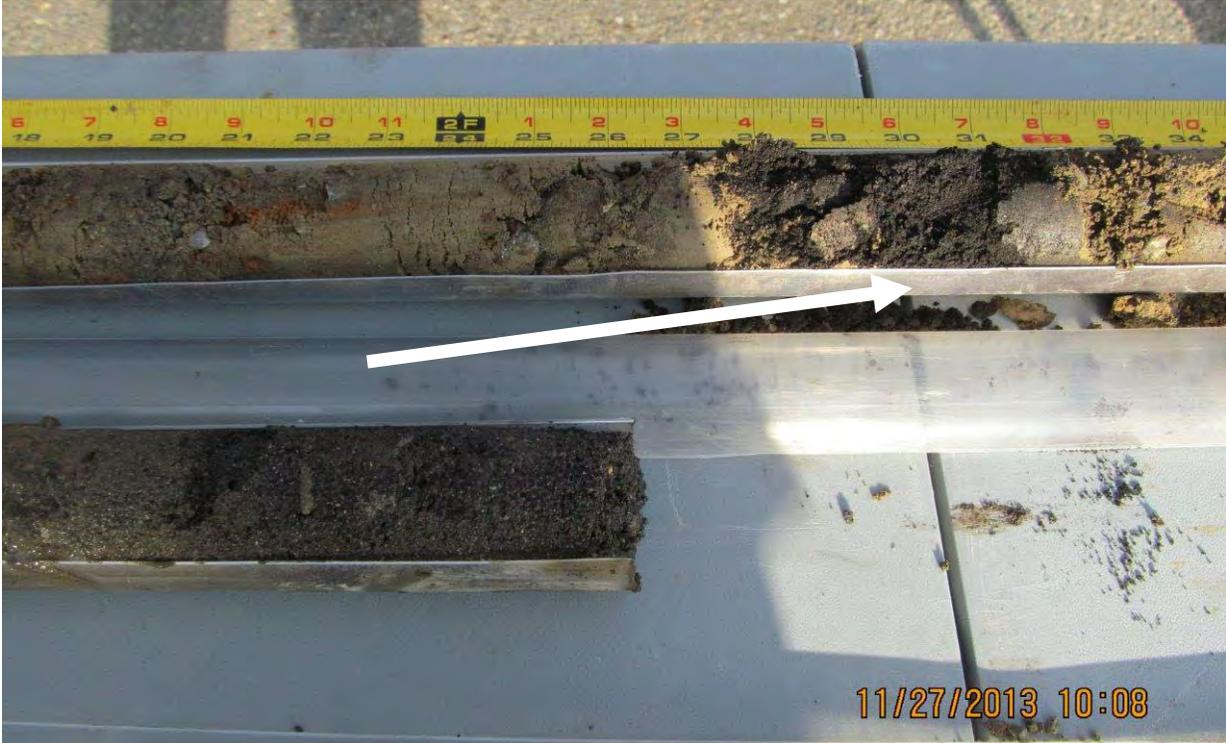
Photo 8. Oily layer from 28-31 inches of borehole 8.
