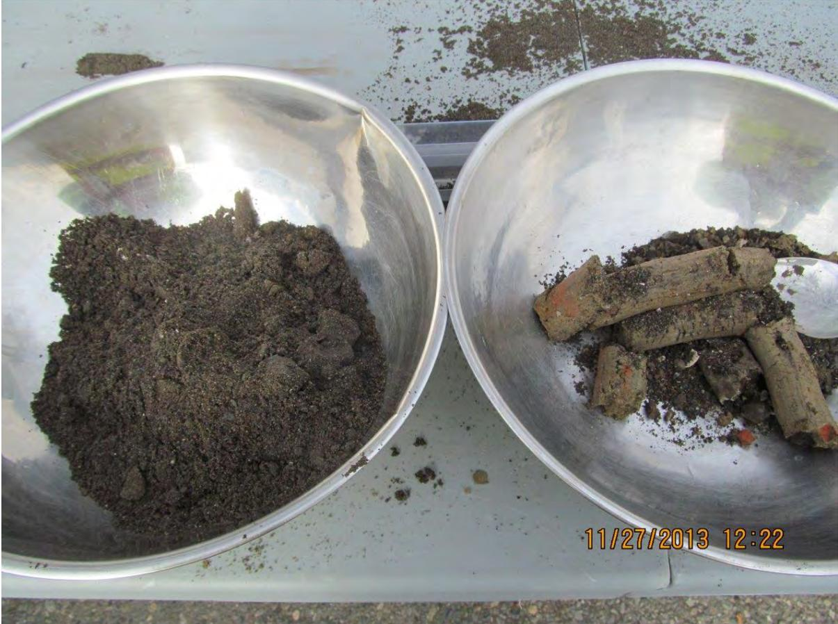
Photo 10. Mixed fill composite (before homogenization) on right (top layer), dredge fill composite on left.
