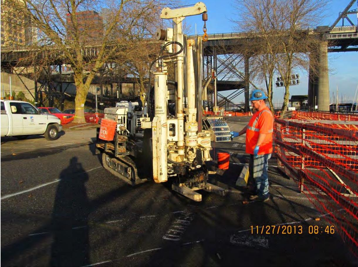
Photo 5. Geoprobe direct push soil corer.
