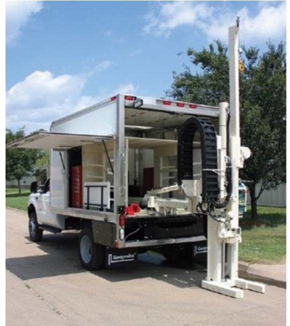
A typical drill rig used for soil air testing.
