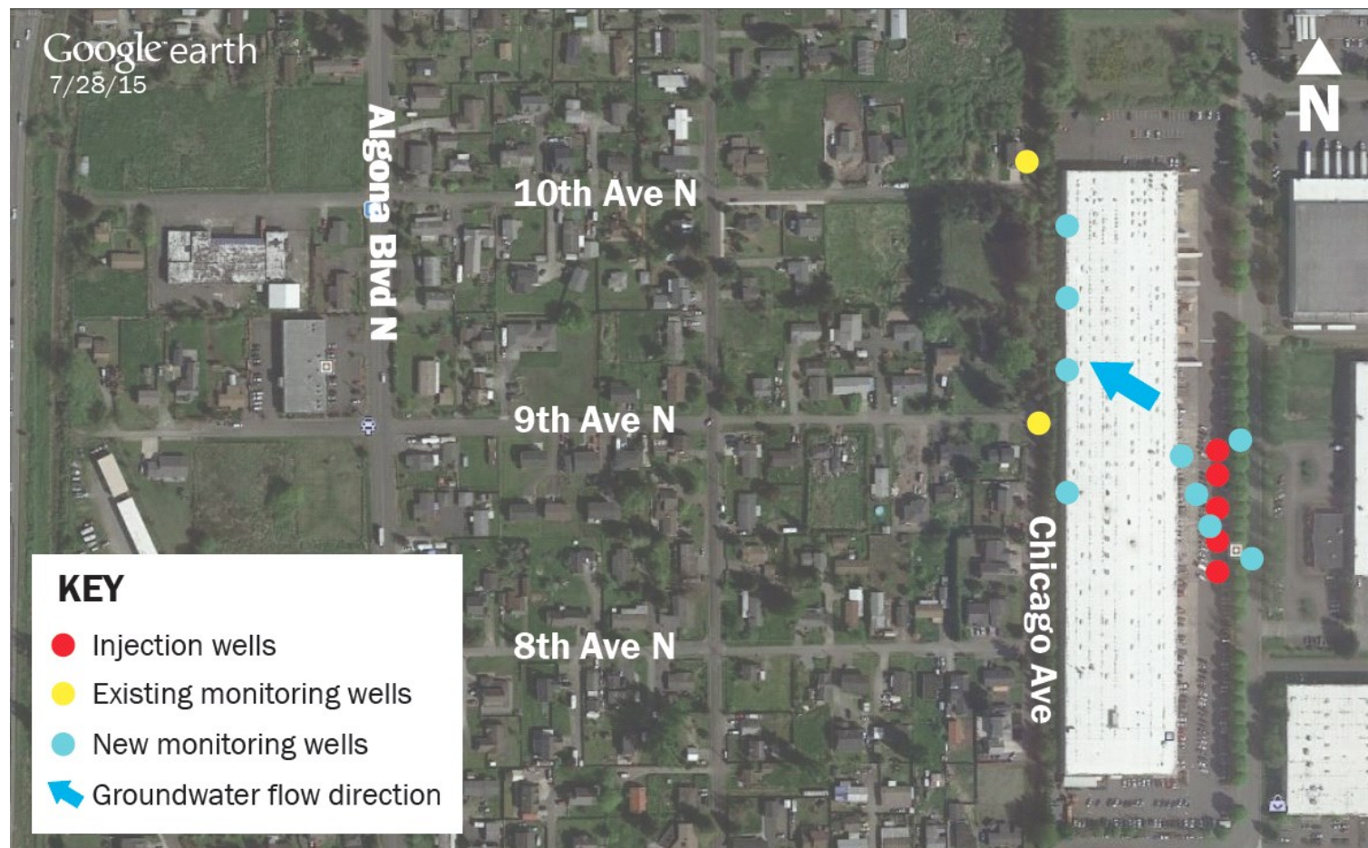
Map of pilot study area, with groundwater monitoring and injection well locations.
