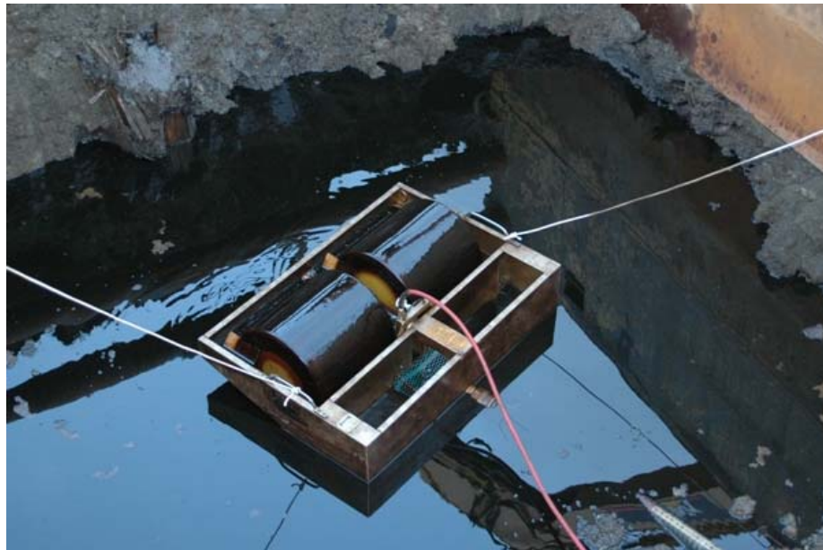
Photo 6. Rotary drum skimmer in operation
