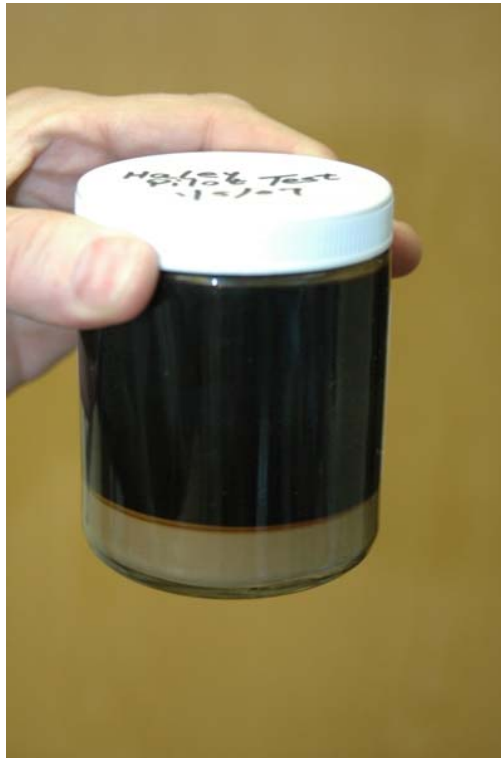
Photo 13. Oil and sediment-laden water recovered during field pilot test
