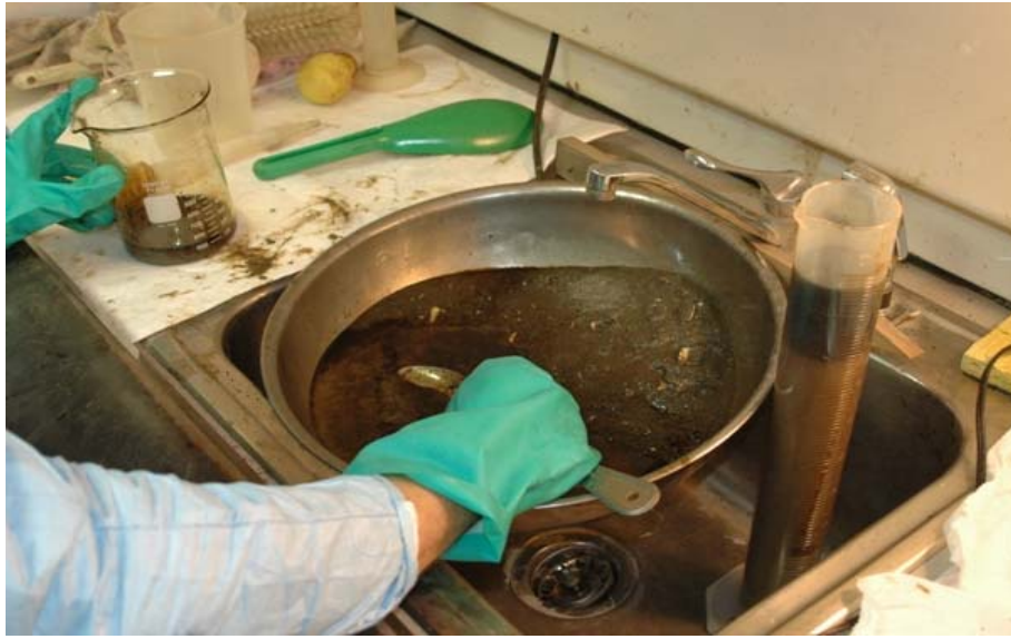
Photo 17. Removal of liberated oil from water surface in mixing bowl.
