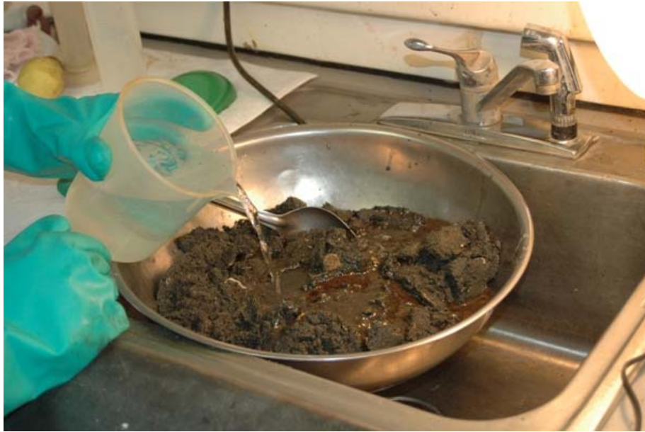
Photo 15. Addition of water to soil prior to bench-scale agitation
