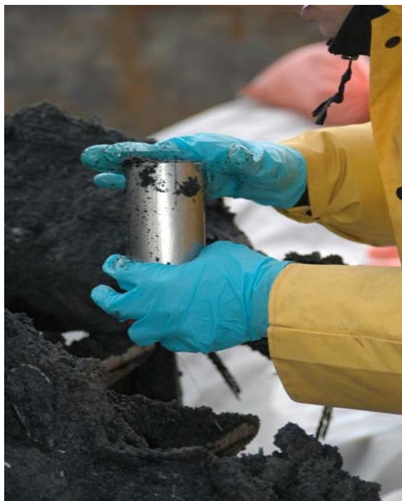
Photo 4. Preparation of soil sample for free product mobility testing
