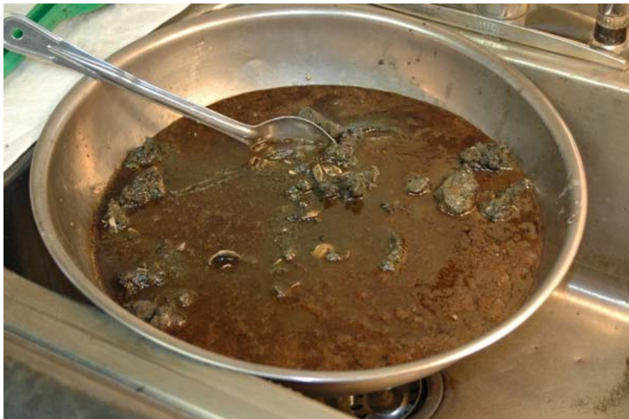
Site Photo 16. Agitation of soil with stainless steel spoon
