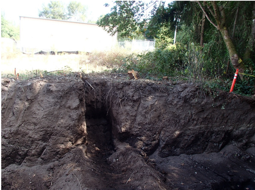
Photograph 14. Test pit in northern side of the South Ditch to delineate contamination
