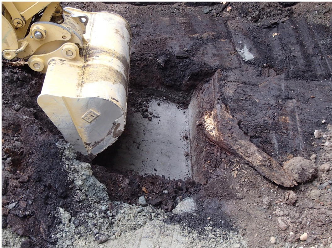
Photograph 12. Test pit in bottom of South Ditch showing clean material underlying woodwaste
