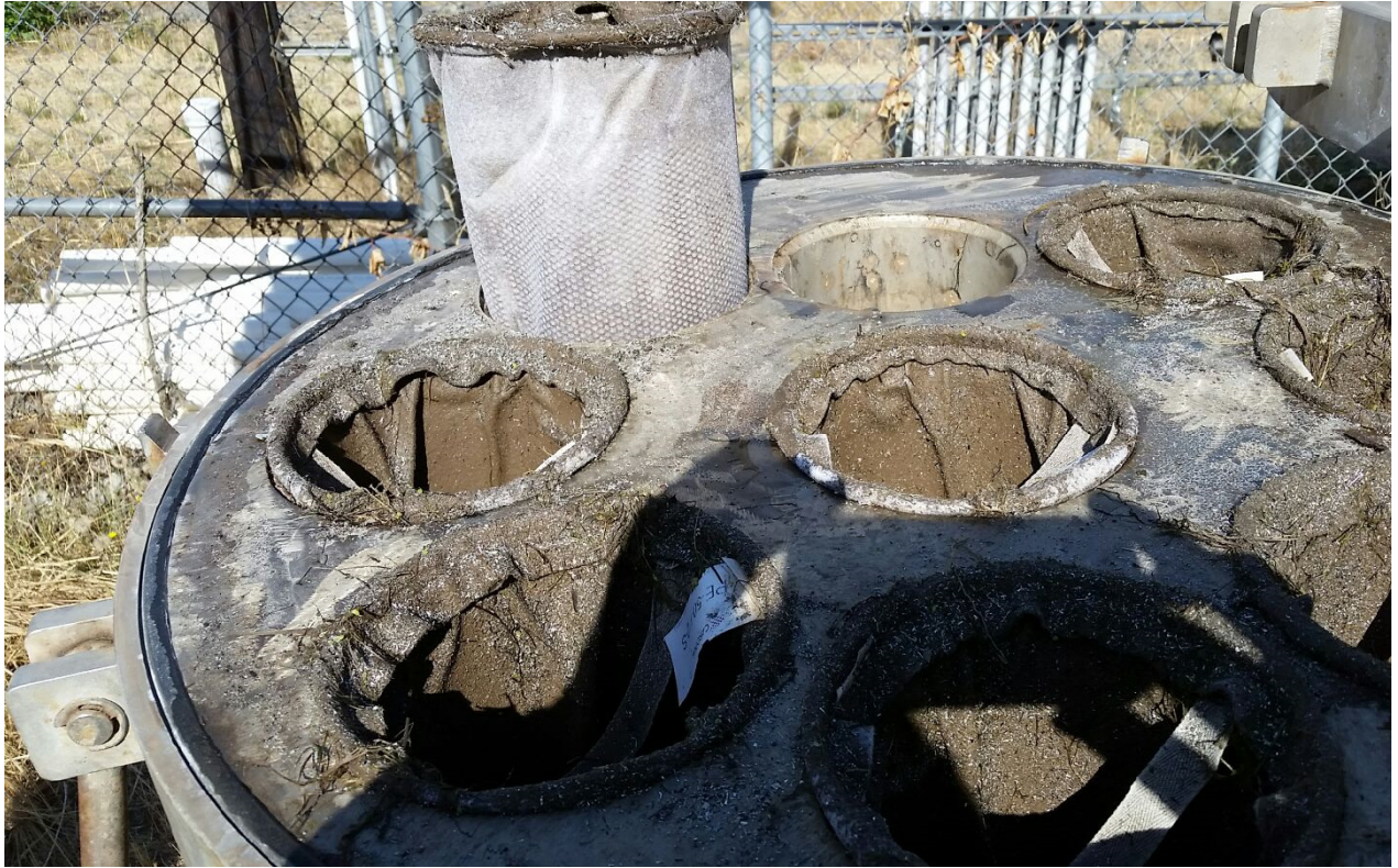
Photograph 17. Metal shaving in filter housing
