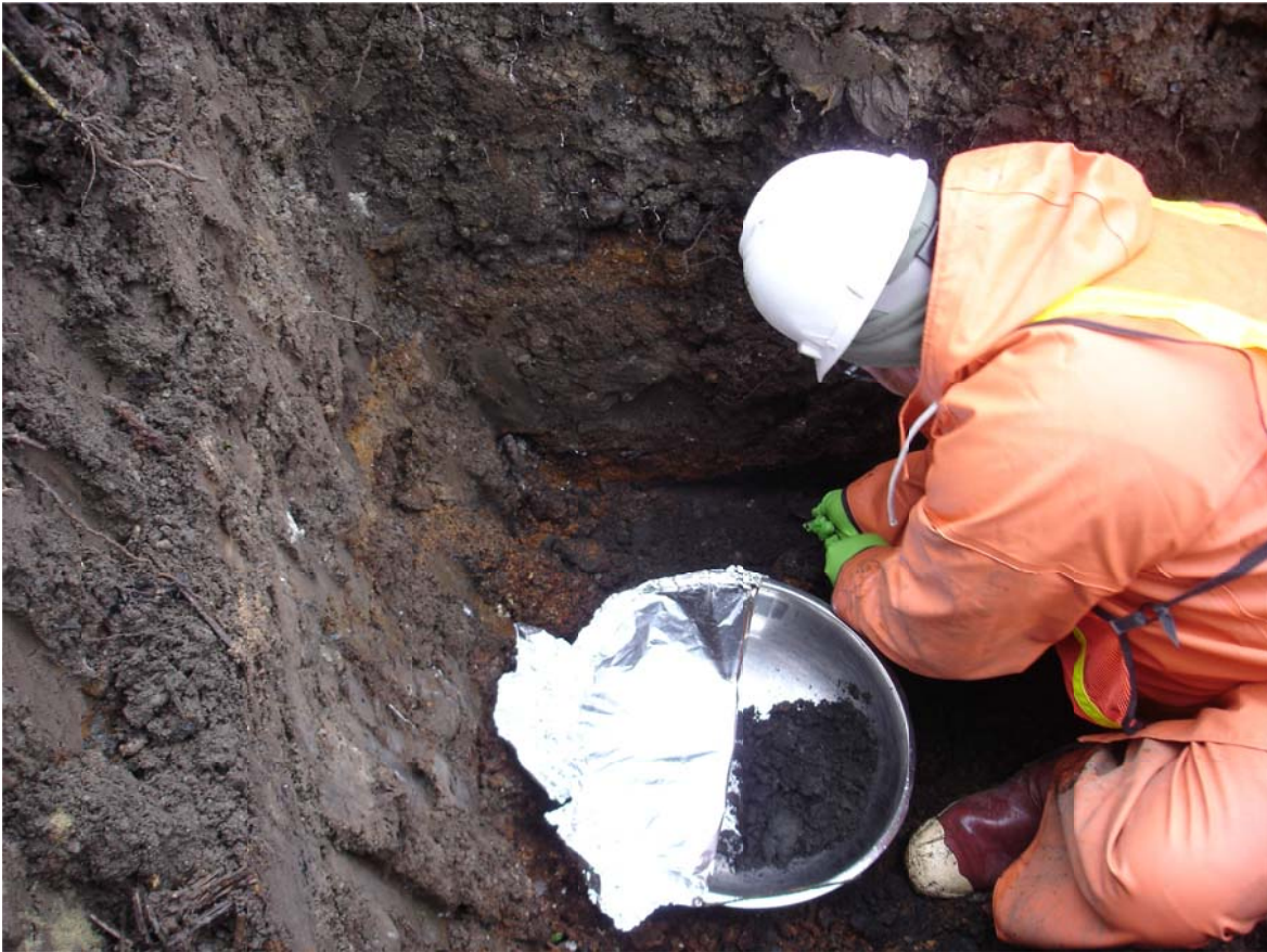
TP-23 Sampling at 4 ft bgs
