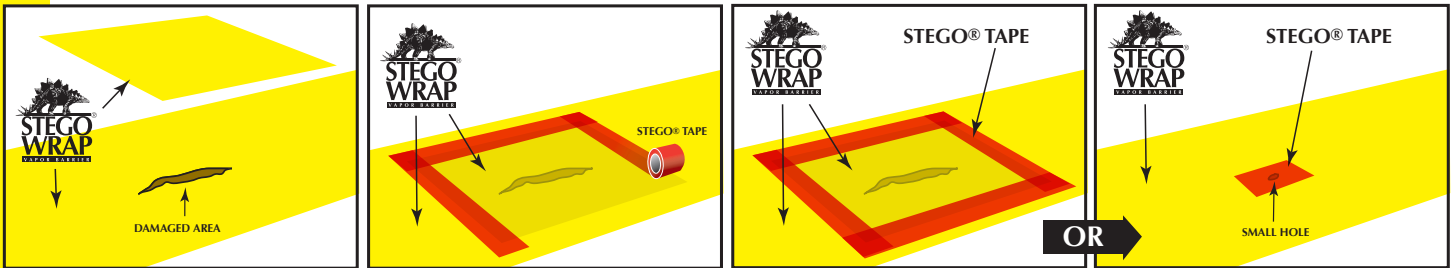
FIGURE 3: SEALING DAMAGED AREAS
