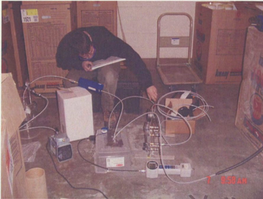
Sub-slab sample location V-4 – Sub-slab Sample Purging setup
