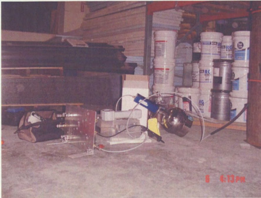
Sub-slab Sample Location V-2 – Sampling Set up
