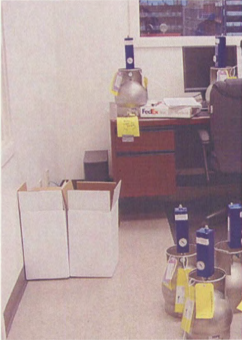
Indoor Air Location IA-5 Setup (canisters staged on the floor in the foreground and on the right side of the desk)
