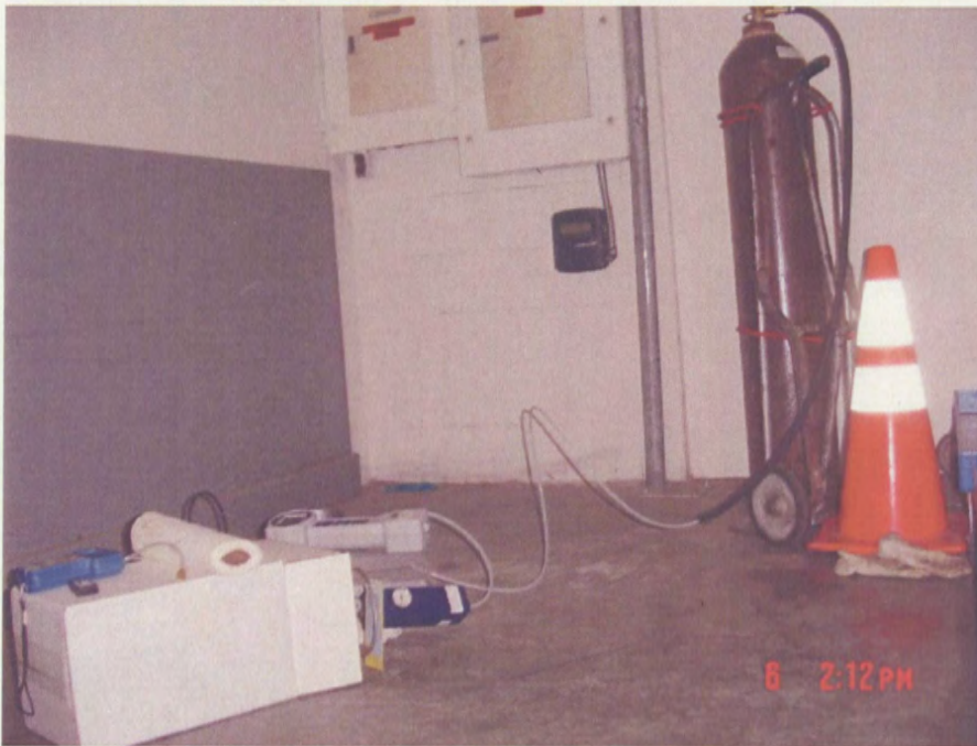
Sub-slab Sample Location V-5 – Sub-slab Sample Collection Setup
