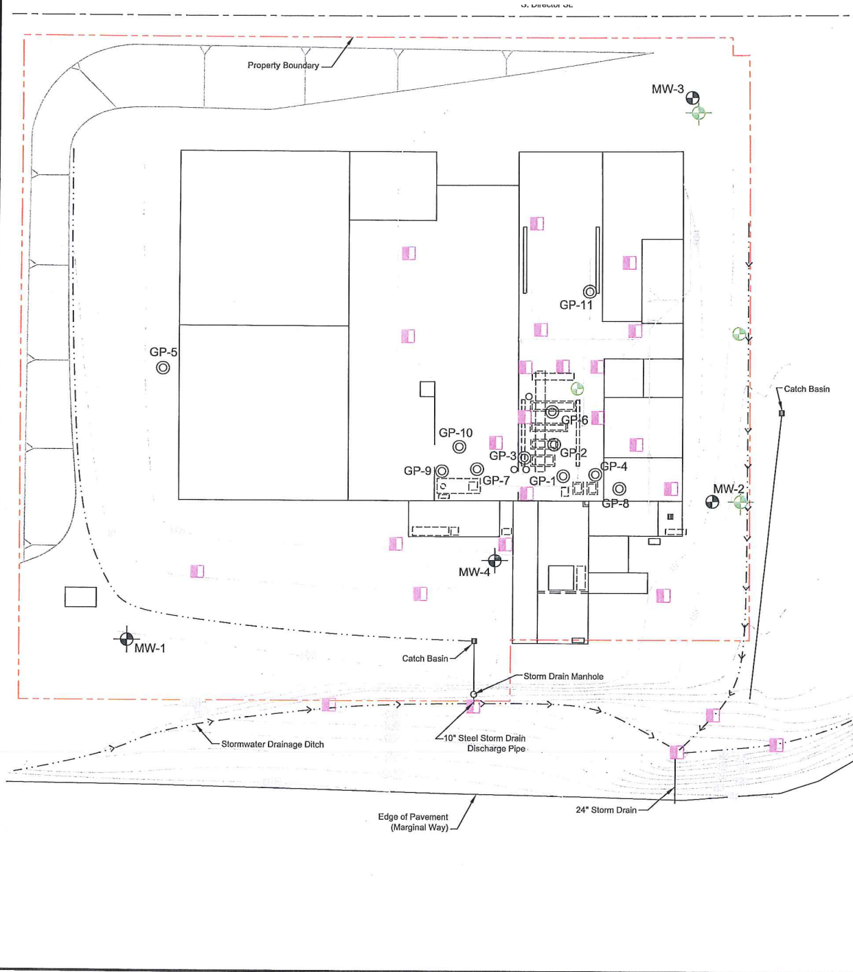
Figure 3 Existing and Proposed Borings and Monitoring Wells
