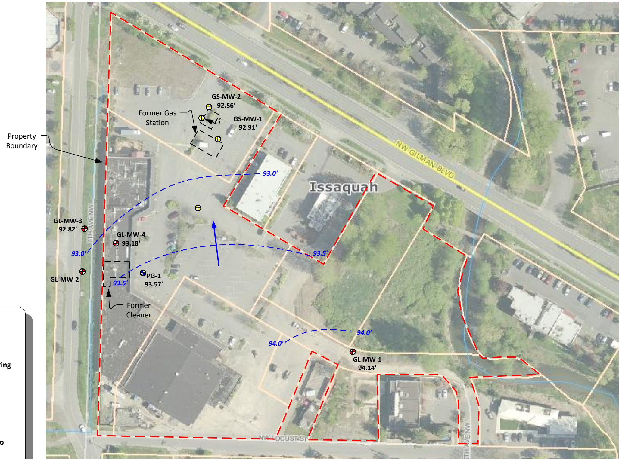
Site Diagram, Groundwater Contours Gilman Square 615 Northwest Gilman Blvd Issaquah, Washington
