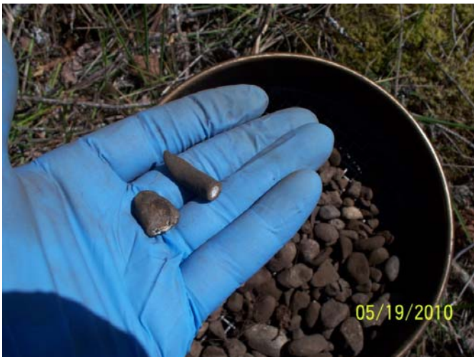
PHOTO 3 Slugs retained on the ¼-inch sieve at Range 62/67, Grid 10-23
