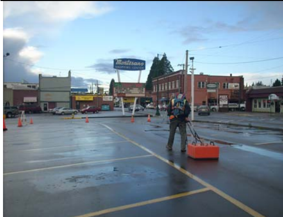
Photo #3: View of geophysicist conducting a ground penetrating radar survey to identify locales of potential abandoned fuel tank at the north-central area of the Site (former Boyer Phillips gas station).
