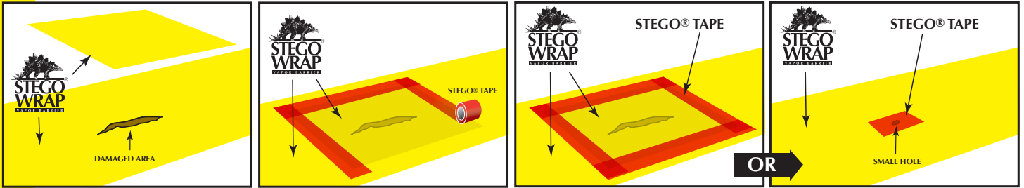
FIGURE 3: SEALING DAMAGED AREAS
